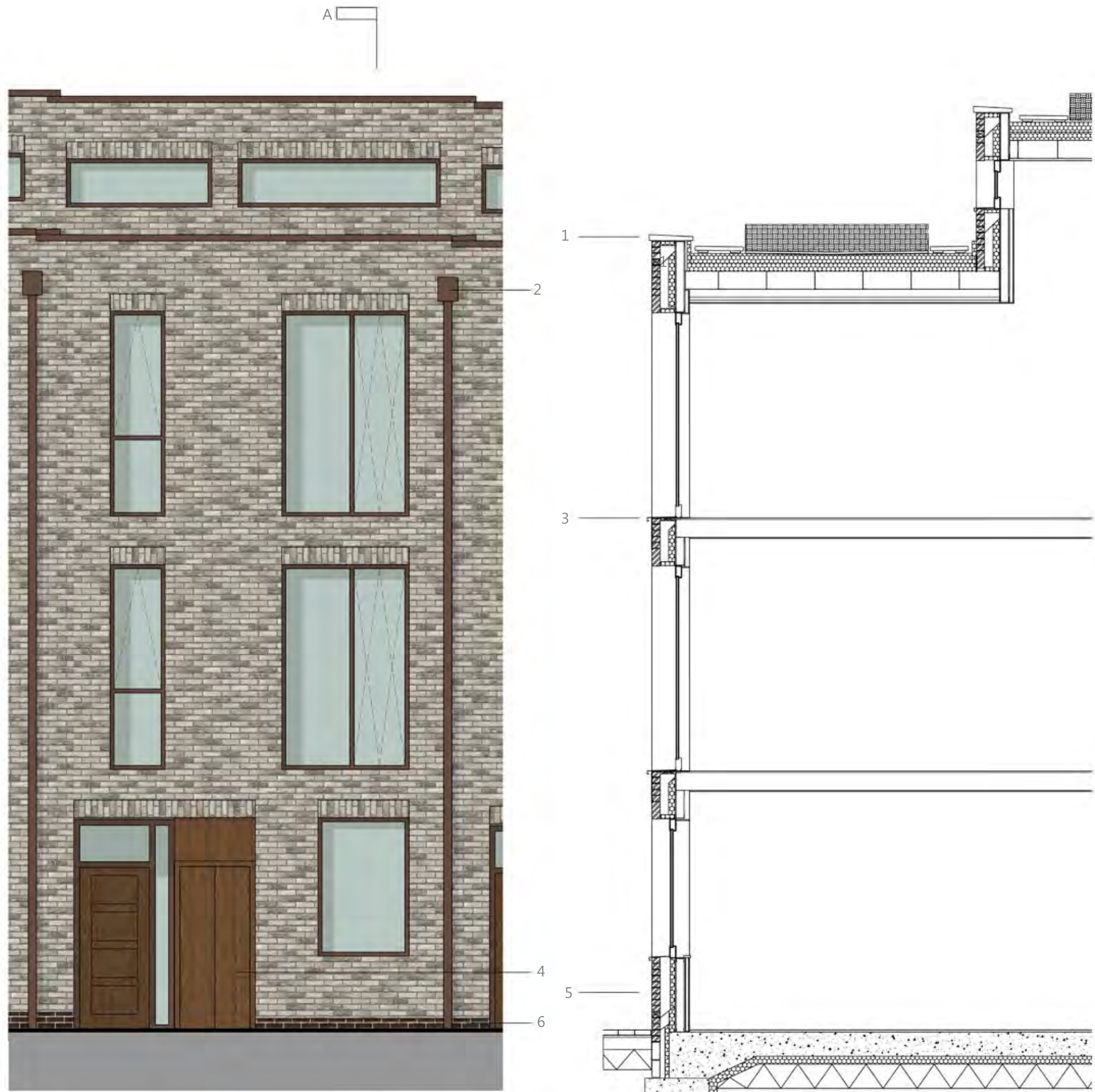
TOWNHOUSE FRONT ELEVATION SCALE - 1:50
