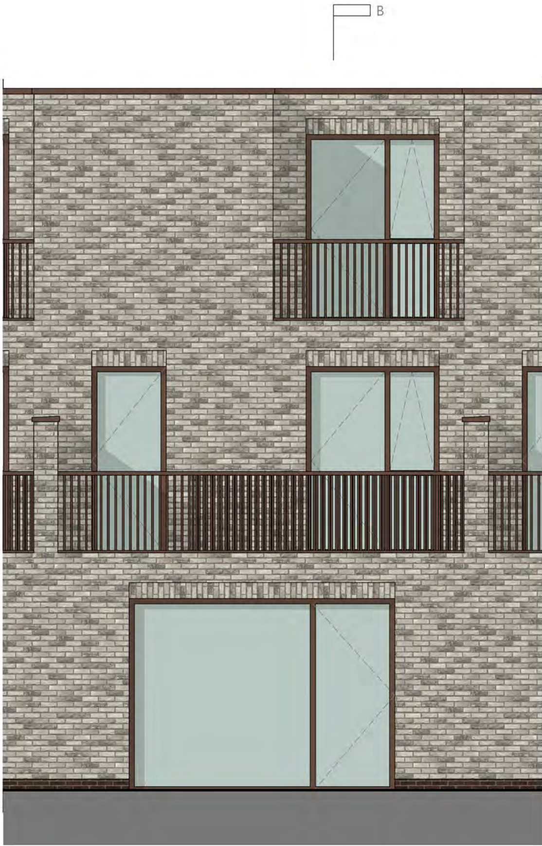
TOWNHOUSE REAR ELEVATION SCALE - 1:50
