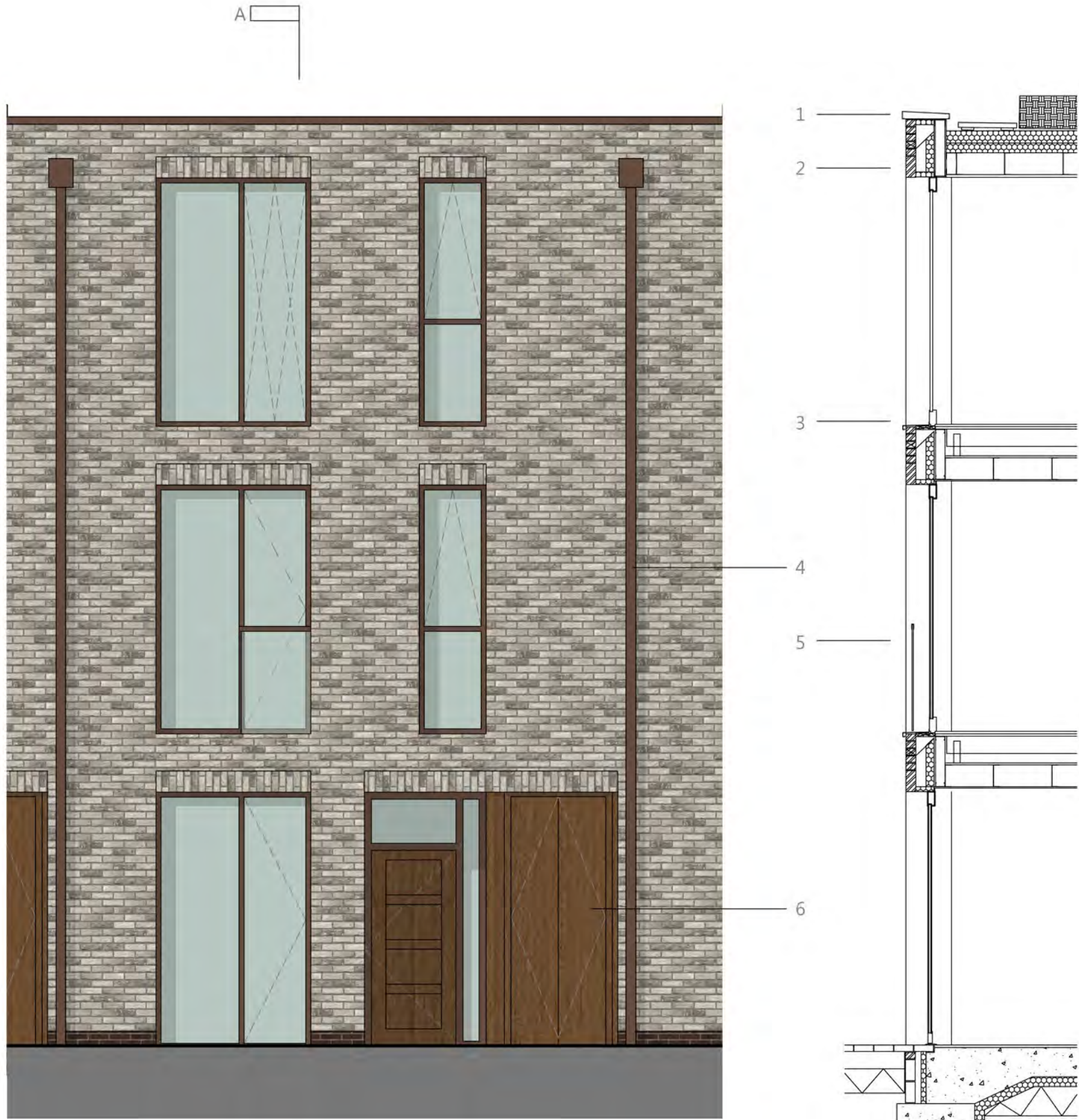
TOWNHOUSE FRONT ELEVATION SCALE - 1:50
