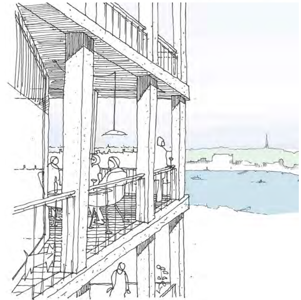
Structural screen contains the balconies within the envelope of the building whilst maximising views and daylight entering the apartments.
