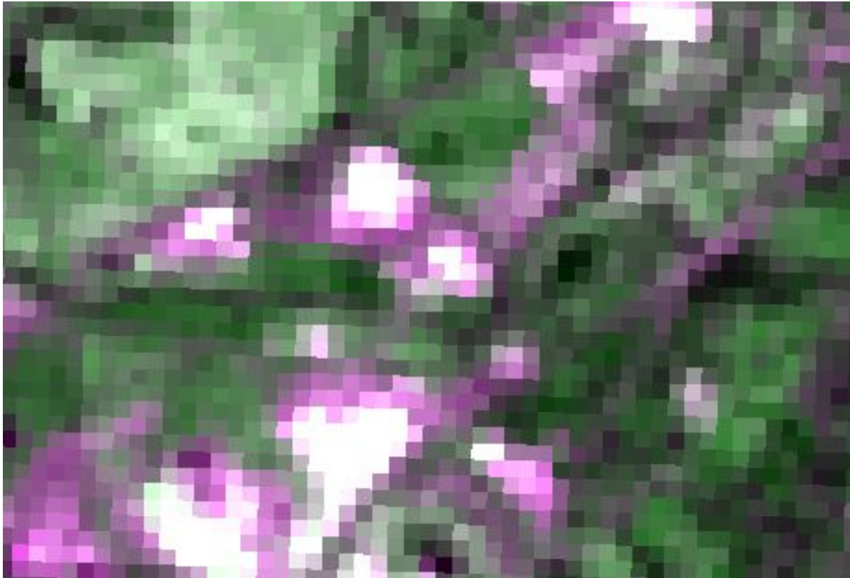
Portion of a Landsat image - you can see individual pixels. Each pixel represents an area 30 meters by 30 meters on the surface of the earth
