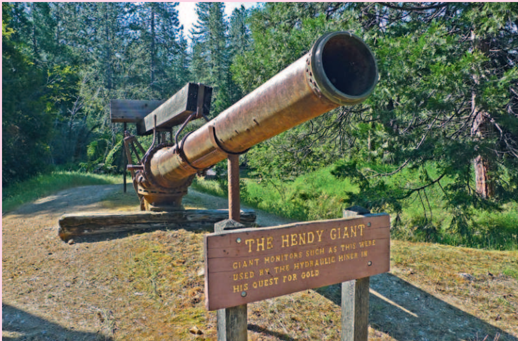
Plate 2.4 Water monitors used at Malakoff Diggins
