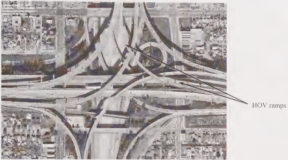
Figure 14.3 I-110 to I-105 interchange in Los Angeles, showing dedicated HOV ramps
