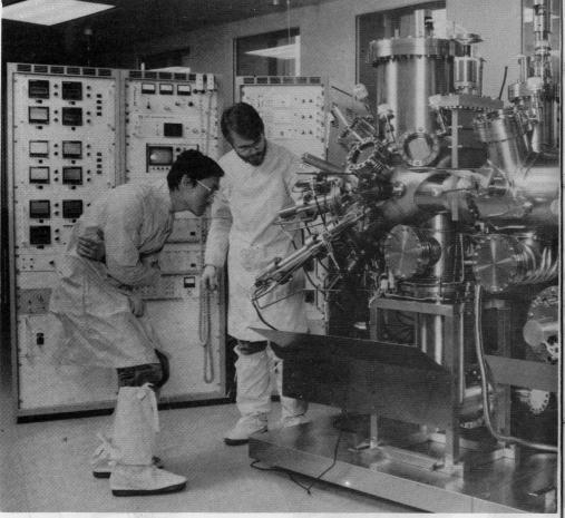
Usually, a number of separate ovens are used, each providing a beam of different material and with mechanical shutters to control the flow. In the midst ensure an even coating.
