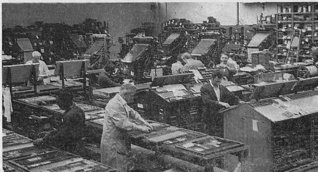
ABOVE LEFT: The pages of type, etc., are being set in their frames for printing, in the background are some of the linotype machines.
