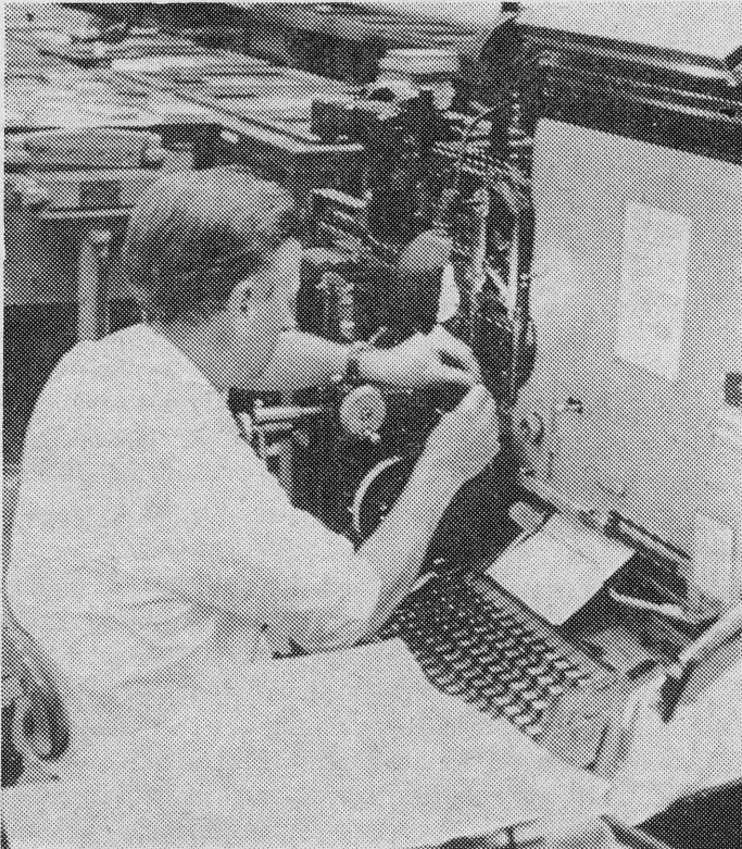
This photo details: the magazines at the top of the machine. These hold different sizes in of type in BOLD , ROMAN and ITALIC . The storage galley containing some twelve lines can be seen bottom left.
