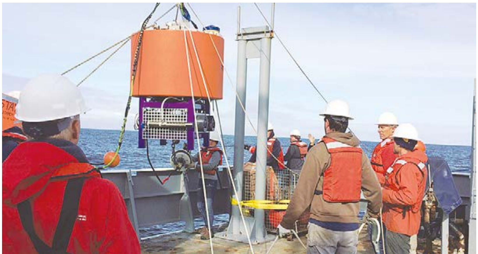
The Environmental Sample Processor being deployed in open water. Photo Credit: NOAA National Ocean service
