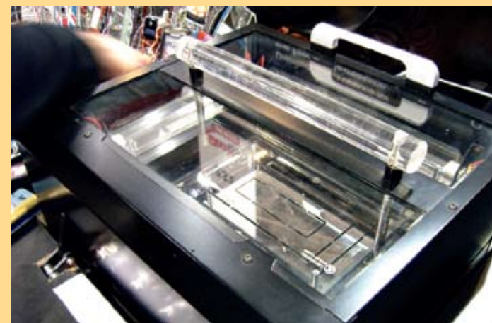
2. DIGISKIN vacuum-forms the printed foil over your gadget.
