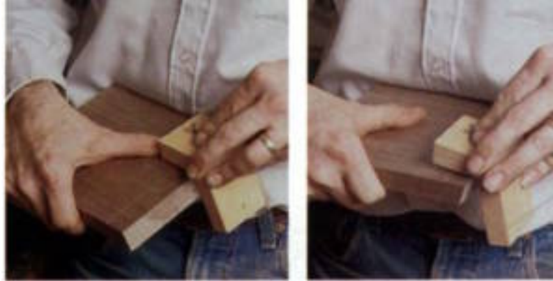
A shopmade marking gauge makes it easy to scribe lines for the pin and tail depth. Two blocks are glued and screwed together at the angle of the stool's joint and a nail scribes the line. The gauge's obtuse angle makes it possible to mark the same distance from the end on both sides of the board.
