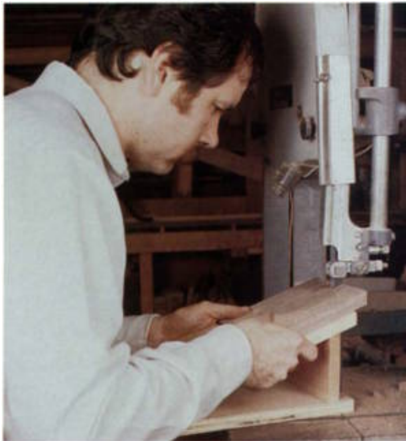
The author bandsaws most of the waste from between the pins using a pitchboard to support the leg at a 19° angle. The pitchboard can also be used to saw the tails on the stool's top board by removing the stop block that's screwed halfway up the ramp.
