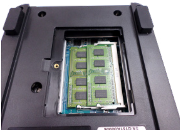
Adding memory modules to your NAS can be a simple performance upgrade.
