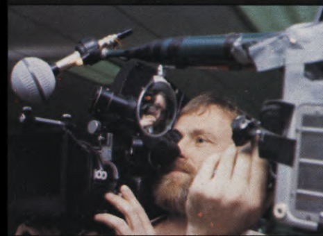
(LEFT) Wide-angle mirror on sound rig allowed 360° view during shooting in tight quarters. Light at end of boom allowed slate marks to be obtained by camera without panning 180° to see digital numbers on sound rig itself. Cameraman's left eye can see top of lens through black tube, which is a diopter/mirror periscope. (CENTER) Elfstrom and Phenix film interview with five-year-old boy at home after 20-hour brain operation which saved his life. (RIGHT) Three-man crew films doctors on daily "TV Rounds", which allowed viewers to get to know patients.
