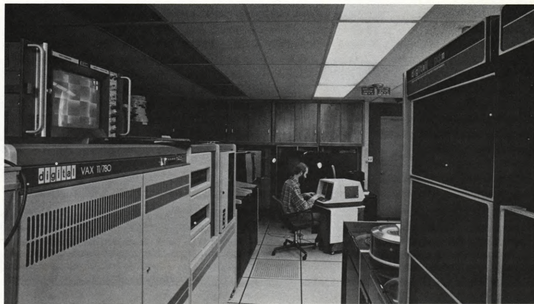
FIGURE 2a —Schematic diagram of the Computer-Assisted Animation System (CAAS). (BELOW) FIGURE 2b —The Digital VAX-11/780 computer (left) has the most strenuous data processing task in the CAAS, assembling the background image and one or more levels of character images into a complete frame for recording on video tape or photographic film. One of the PDP-11/34 minicomputers controlling animation stations can be seen at right. (NOTE: The author, Dr. Catmull, formerly Director of the Computer Graphics Lab at New York Institute of Technology, is currently Director of Computer Systems Development, Lucasfilm Ltd., San Anselmo, Calif.)
