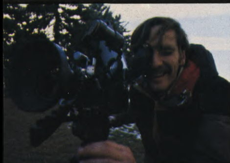
(LEFT) Dater lines up a short, using the Sachtler tripod. All zoom lenses were fitted with fluid collars for smoother zoom action. (CENTER) Zeiss High-speed Distagon T/1.3, 9.5mm lens was responsible for ability to shoot without lights. Crew obtained the first one to be privately owned in the United States. Modified footage scale facilitated quick focusing in low light, through an arrangement of mirrors and diopters. (RIGHT) Elfstrom and Phenix film, as unseen accident victim explains events which brought him to hospital.
