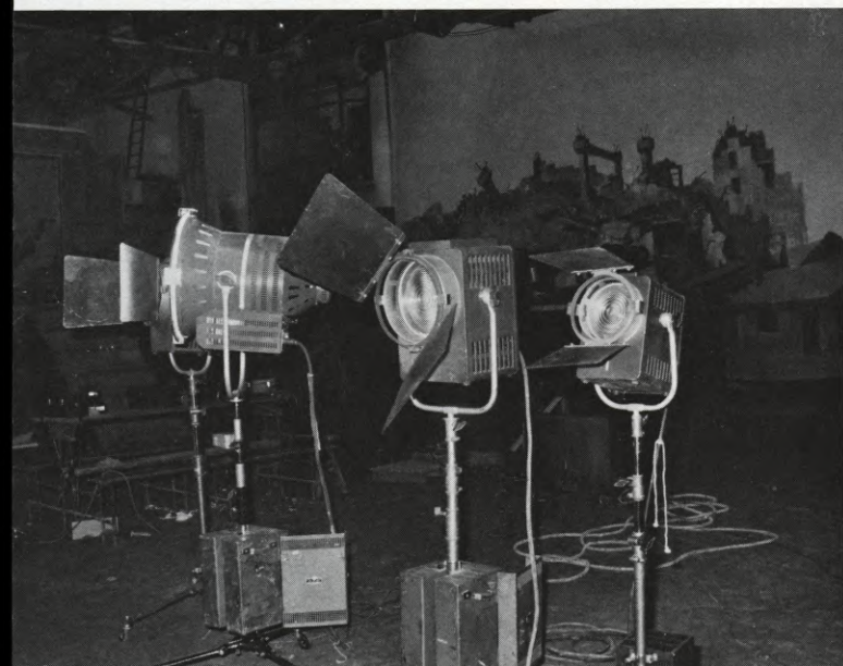
(LEFT) Experimental HMI-type lights. From left to right: 4000 watts (non-fresnel), 2500 watts and 1200 watts. Note the small size of the ballasts, which are relatively lightweight. All are operated on D.C. and are "flicker-free." (RIGHT) Solid-state electronics dimmers used for the control of lights and dimming in the Shanghai Television Studios.
