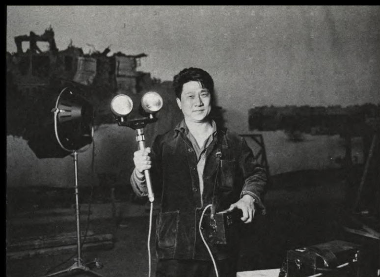
(LEFT) Mr. Yang Chung-fang of the Research Group of Light Sources of the Shanghai Film Studio demonstrated the battery-operated dual-HMI-type light. Note the small size of the battery and ballast. (RIGHT) The music and singing for the Peking Opera were recorded on the optical track of sprocketed 35mm film then played back on stage during shooting. The performers were filmed as they played in synchronization to the music, in standard "playback" fashion.
