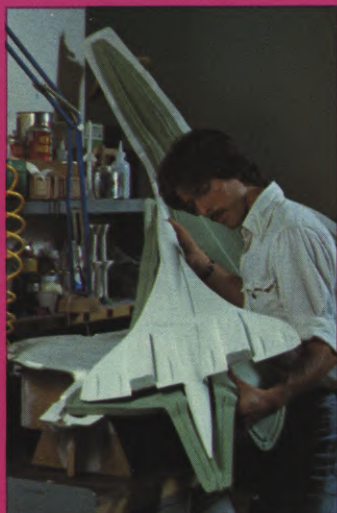
(LEFT) Modelmaker Sean Casey removes cast epoxy Concorde model from rubber glove mold, which reproduces much of the fine detail, as well as the exact form, of the original. (CENTER) Color wedges being finalized by Milrad. (RIGHT) Finishing touches are applied to sketch of Phantom jet, which will serve as guideline for detail work. (BELOW RIGHT) The final product of all the blood, sweat, tears and energy expended: portion of a blown-up frame showing the graceful Concorde speeding through the clouds (with nary a trace of yellow or wires).
