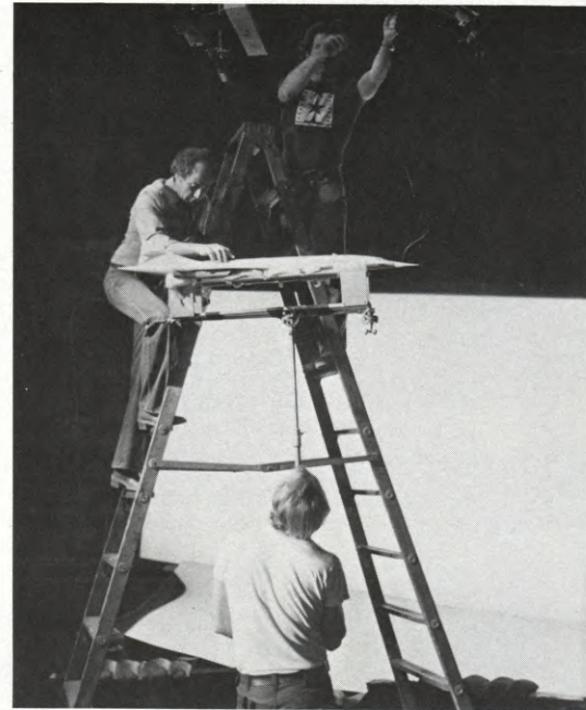
Concorde model is suspended from a rig allowing for simultaneous changes in roll, pitch and yaw attitudes, as well as rotation and arc movements.
