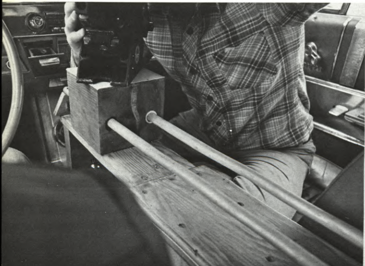
(LEFT) FIGURE 3—In another view of the track with the extension, one can see the forwardmost position of the camera. (RIGHT) FIGURE 4—Here, with Director Gary Walkow behind the camera, the track spans the rear armrests, allowing for the execution of lateral camera moves.
