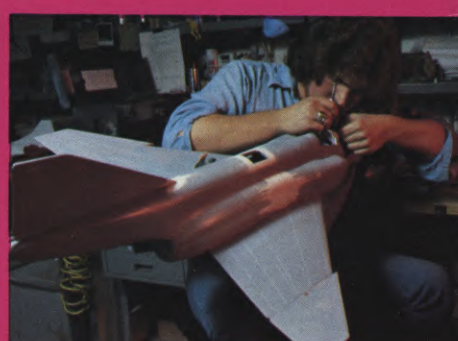
(LEFT) Chief Modelmaker Pete Gerard uses lacquer tough-up gun to spray special yellow primer onto the Concorde. (CENTER) Gerard uses high-strength filler to bring about subtle changes and repairs on the surface of the Concorde. (RIGHT) Detail wizard Ken Larson with a nearly completed Phantom model. (BELOW LEFT) The crisp scribe lines had to be constantly maintained throughout the finishing stages of each model. Here Mike Joyce attends to a tiny detail. (CENTER) Every detail was carefully scaled from original photographs and drawings. Pete Gerard outlines a landing gear cover flap. (RIGHT) Modelmaker John Curtis installs miniature pilot figure in F-4 Phantom model.
