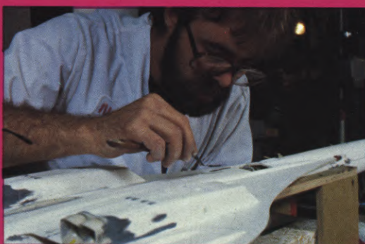
(LEFT) Chief Modelmaker Pete Gerard uses lacquer tough-up gun to spray special yellow primer onto the Concorde. (CENTER) Gerard uses high-strength filler to bring about subtle changes and repairs on the surface of the Concorde. (RIGHT) Detail wizard Ken Larson with a nearly completed Phantom model. (BELOW LEFT) The crisp scribe lines had to be constantly maintained throughout the finishing stages of each model. Here Mike Joyce attends to a tiny detail. (CENTER) Every detail was carefully scaled from original photographs and drawings. Pete Gerard outlines a landing gear cover flap. (RIGHT) Modelmaker John Curtis installs miniature pilot figure in F-4 Phantom model.
