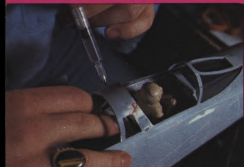
(LEFT) Ethylene dichloride is being injected into a seam to bond thin layers of polystyrene to the inside of the cockpit. Most of these aircraft models included meticulous detail, even to the pilot's switches and instruments. (CENTER) The special filming rig mounted from the ceiling on Stage Four of Universal Studios Special Effects Facility. (RIGHT) The rig, seen in the mirror on the left hand side of this photograph, with its electronic drivers being tested by Assistant Cameraman Chuck Schumann.
