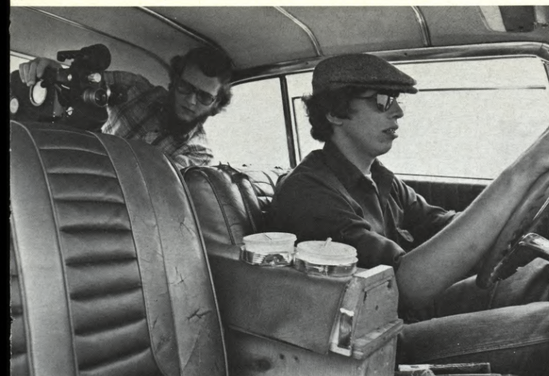
(LEFT) FIGURE 5—With Gary Walkow and C.M. Heard we see the canopy disguise covering the front eighteen inches of the track, which would otherwise be visible to the camera when its 10mm lens is pointing towards the windshield. (RIGHT) FIGURE 6—When the camera is moved forward—in this case, into a profile of the driver—the canopy is pushed forward towards the dash.
