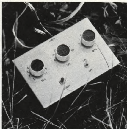
(ABOVE) Electronic timing box which controlled the Beaulieu single-frame, time-lapse system. (RIGHT) Single-frame solenoid device for use on the Beaulieu. Both devices were "homemade".
