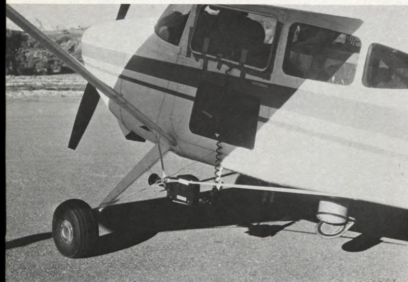
(ABOVE LEFT) Close shot of the 16mm Beaulieu camera in its Sea Research and Development plexiglass underwater housing. This rig not only works extremely well for underwater work, but is considered a bit more expendable than the more expensive camera equipment on the shoot. (BELOW LEFT) Photosonic camera mounted to Cessna footstrut for filming of Greenback Trout planting sequence. (RIGHT) A closer look at the mount, which was built for filming dives on the lake.
