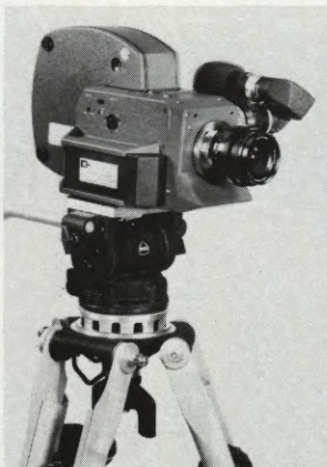
Ultra T 25mm (T1.25) prime lens shown with "state-of-the-art" GSMO 16mm camera (with 400' quick-change cassette-type coaxial magazine), CP orientable viewfinder and Universal 16FX fluid head tripod.
