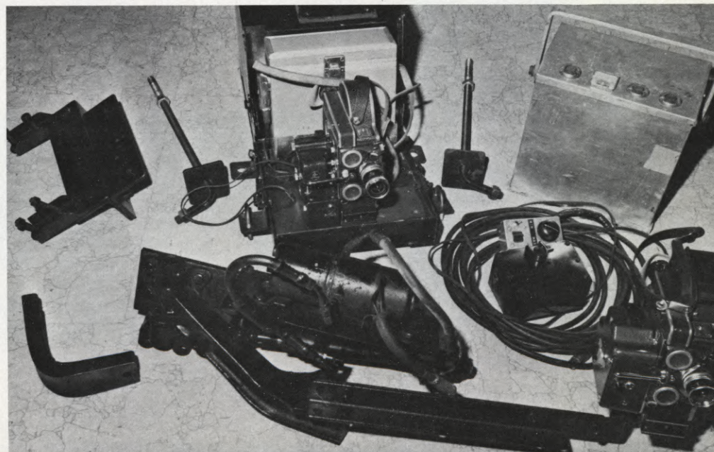
Custom-designed and built camera mounts used on the steam locomotive, clockwise: (a) Bracket used to film closeup of engineer, (b) Adjustable angle mount for high position point-of-view of the locomotive, (c) Enclosed mount with cover, used for front locomotive point-of-view, (d) 12-volt power supply for control relays and hydraulic camera mount, (e) 12-volt controls, (f) Hydraulic camera mount.
