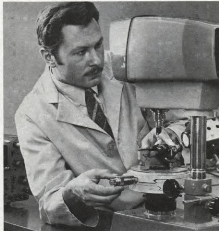
Checking critical relationship between claw and register-pin on 16mm ARRI movement. Tolerance is 0.0004 inch. Screen image is magnified ten times.
