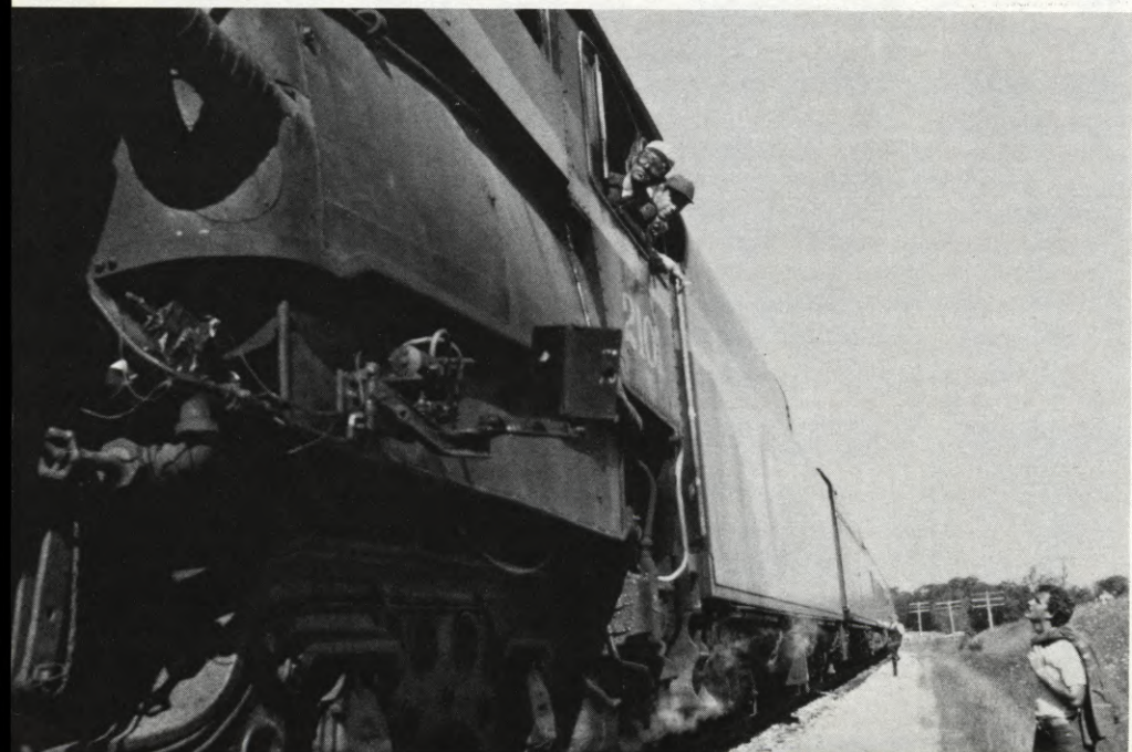
Locomotive of the steam-powered, 20-car "Chessie Steam Special", which operated during the seasons of 1977 and 1978 to celebrate the B & O Railroad's 150th Anniversary. Note the motion picture camera mounted above the coupler to shoot "locomotive point-of-view" shots. (BELOW) The ingenious hydraulic camera mount located on the side of the locomotive for filming men "driving" the train.
