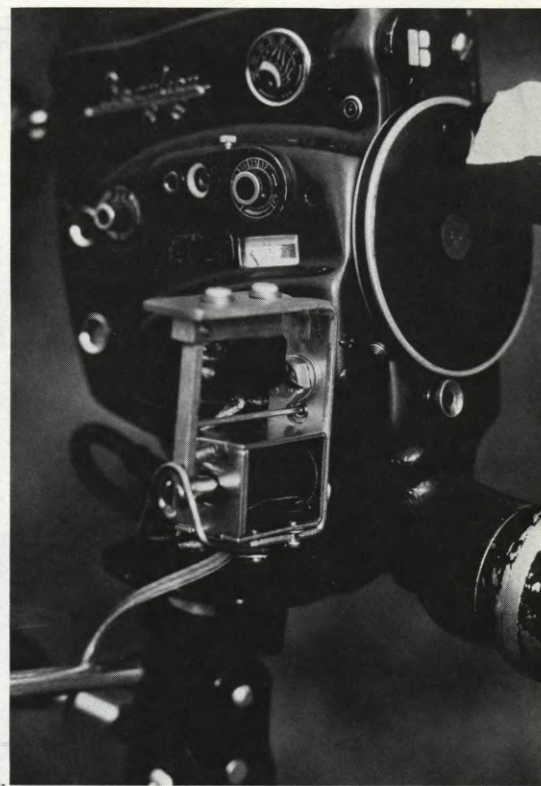
(ABOVE) Electronic timing box which controlled the Beaulieu single-frame, time-lapse system. (RIGHT) Single-frame solenoid device for use on the Beaulieu. Both devices were "homemade".
