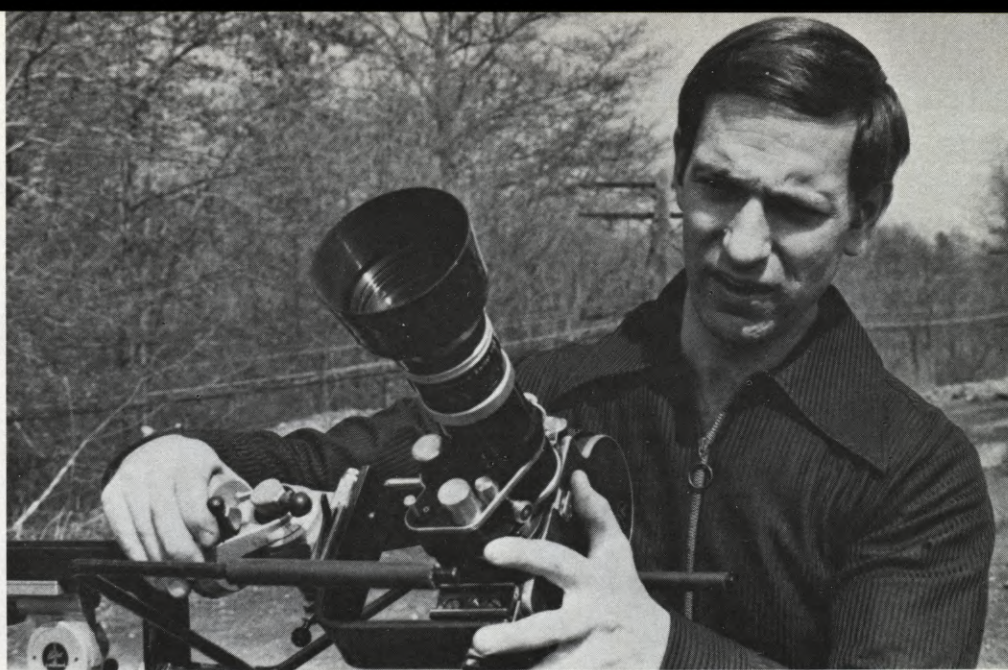
Checking the position of the end-of-travel "stops" used in flip shot where camera is tilted 180 degrees as train passes. The stops are the two rubber-covered rods in front of and behind the camera. The camera is fastened to a horizontally placed panhead (which the operator holds in his right hand in this photograph).
