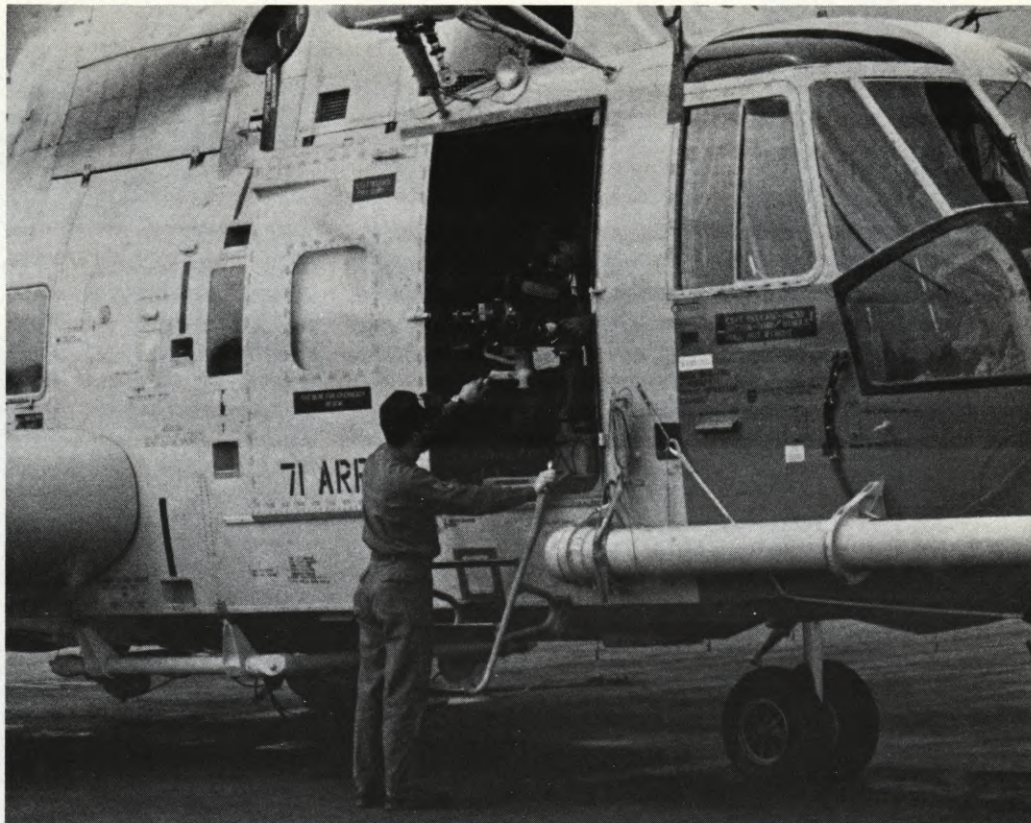
The Tyler Mini-Mount was set up in an Air Force HH-3 helicopter for aerial cinematography. A special advantage to Air Force motion picture crews is the available use of airplanes and helicopters for filming.
