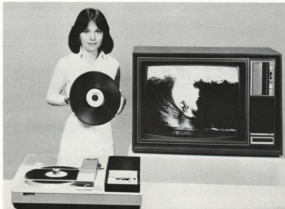
The new "VHD/AHD" grooveless, capacitive pick-up Video Disc System, developed by the Victor Company of Japan, Ltd., plays a 12-inch grooveless plastic disc which contains up to a total of two hours (both sides) of color programs with sound. The player is also capable of playing digitally recorded super hi-fi audio (PCM) discs, also developed by JVC. The player connects to an ordinary domestic color TV receiver.
