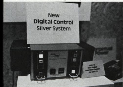
(LEFT) New Anton-Bauer Digital Control Silver Battery Charger. The battery snaps onto the side of the charger without cables. All charge parameters are precisely controlled by a digital computer circuit. The high-energy silver battery has three times the power density of Ni-Cad. (CENTER) Comprehensive Video displayed the new Sinclair Mini-Monitor TV unit. (RIGHT) Coherent Communications exhibited, among many accessories for the soundman, this PICOMixer, a quality 6-input mixer.
