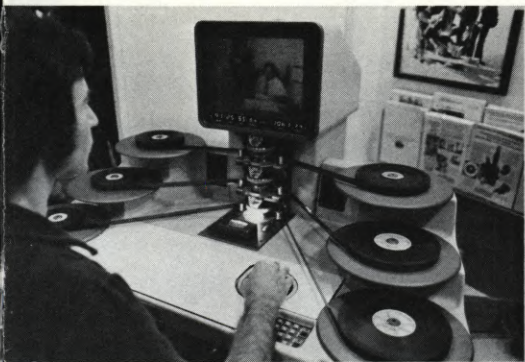
(LEFT) Inventor Robert Olodort at the console of his Cinema Products-built U/F-16 upright-flatbed editing machine. (CENTER) The new Steenbeck series of flatbeds utilize multiple electronic drive motors. (RIGHT) The new Cinemonta editing tables use the unique Optical Crown Imaging System, which employs 24 high-speed lenses instead of a prism. This results in almost twice the normal resolution. A side-by-side comparison of the two systems is impressive.
