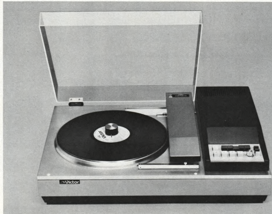
The new "VHD/AHD" grooveless, capacitive pick-up Video Disc System, developed by the Victor Company of Japan, Ltd., plays a 12-inch grooveless plastic disc which contains up to a total of two hours (both sides) of color programs with sound. The player is also capable of playing digitally recorded super hi-fi audio (PCM) discs, also developed by JVC. The player connects to an ordinary domestic color TV receiver.
