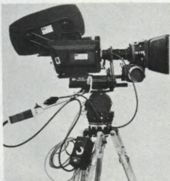
Studio-Rig: zoom control, orientable viewfinder and O'Connor model 50-C fluid head and legs.
