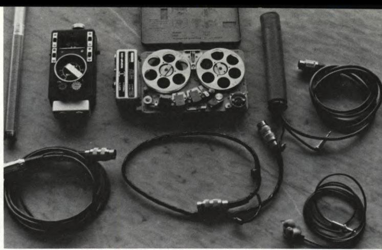
Components of the sound system (left to right): Sennheiser 415 microphone, microphone cable with plastic connectors for light weight, SON manual control unit, Nagra SNN with crystal, leather covered tube containing Gleason's electronic wizardry to start, stop and bloop recorder as the 16SR turns on and off, molded earplug to fit in cameraman's right ear.
