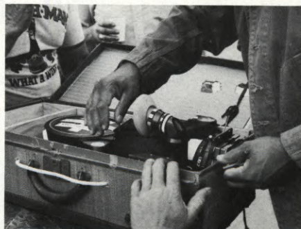
Above: Operator, dressed as migrant worker, checks fit of hole cut in suitcase for 35BL viewfinder. Below: The 35BL being positioned inside the suitcase.
