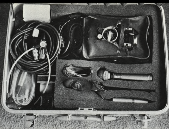
(LEFT) Entire Nagra SNN sound system packs into one #103 Halliburton case, ready to roll. Box with digits at lower left in case is a printed circuit thumbwheel with numbers from 0 to 99, used for slating sound takes. (RIGHT) Arriflex 16SR camera and magazine case custom-fit by Vision Associates into Halliburton #105 cases. The camera is hand-carried everywhere. The lens case can be shipped. Note camera report card on magazine.
