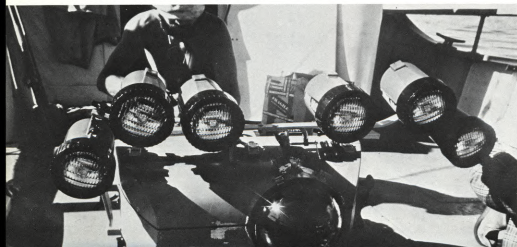
The camera system shown with six underwater portable lighting units mounted on the housing. These were Oceanic PML 100 and 200 lights used for fill during a sequence shot in the murky waters beneath an oil-drilling rig in the Santa Barbara Channel. Each light was 250 watts, with a 2400°K color temperature.
