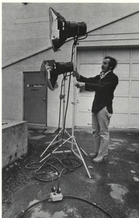
(LEFT) The tie-in apparatus is standardized on two cables and connector sizes, with the main cables looping through receptacle boxes, as shown. (RIGHT) Equipment chosen for the Filmobile is continually scrutinized for replacement on the basis of bulk/performance. The Arri 16SR is compact and highly personal, as well as being a super performer.
