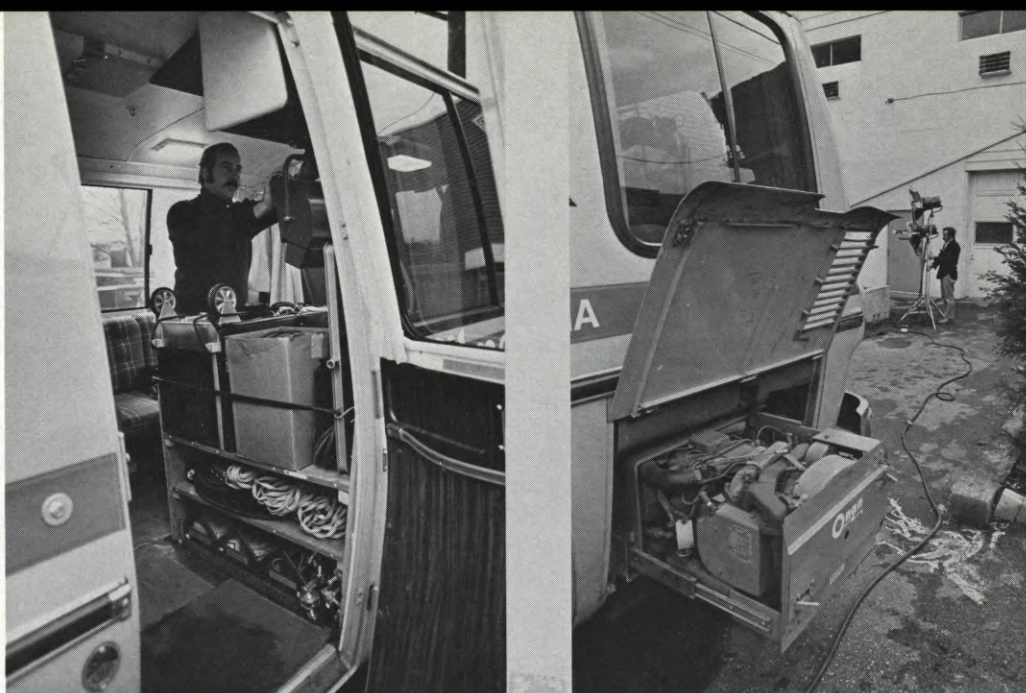
(LEFT) Highest priority lighting and grip equipment is located adjacent to the door. (RIGHT) A two-cylinder, 6KW generator supplies power for daylight fill or modest interior setups up to 100 meters (328 feet) over the Filmobile's standardized cables.
