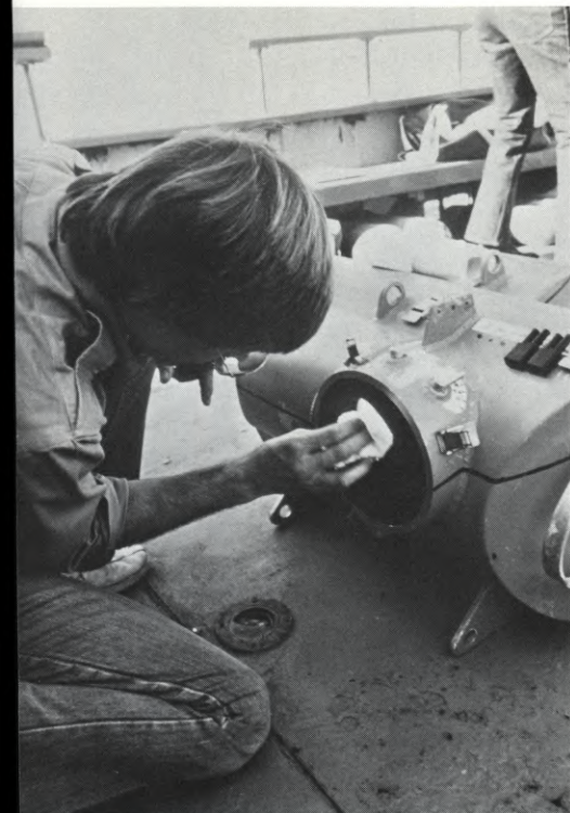
Assistant cameraman Averill Townsend cleans the port of the underwater housing before the camera system is lowered into the water for filming with the extreme wide-angle "fisheye" lens.
