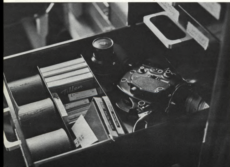
(LEFT) One drawer in the camera department includes color correction and special effects filters, adaptors, lenses and a Beaulieu "grab" camera. (RIGHT) This half of the well-equipped camera department includes three cameras, tool cabinets, accessories cabinet with battery charging area on top, and tripods and heads below. The Filmobile has proved to be highly cost-effective for widely separated location production.
