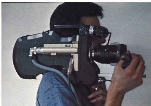
(LEFT) A four-man "portable" video crew shooting the Olympic Games in Innsbruck. Alongside them stands one man with an Arriflex. (CENTER) The Aaton 7 camera, shown equipped with TV viewfinder attachment. (RIGHT) Aaton cameraman with his director, who is holding a small battery-powered TV monitor to check the cameraman's coverage. The Aaton, long in development, represents a high-point in sophisticated camera design.
