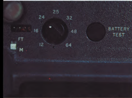
(LEFT) Closeup of the GSMO controls. There are a minimum of controls, making the camera very simple to operate, despite its highly sophisticated electronics. (CENTER) The GSMO camera body, showing the film transport mechanism. (RIGHT) The GSMO 100-foot (30-meter) cassette magazine, with cover removed to show take-up side of the coaxial mechanism.
