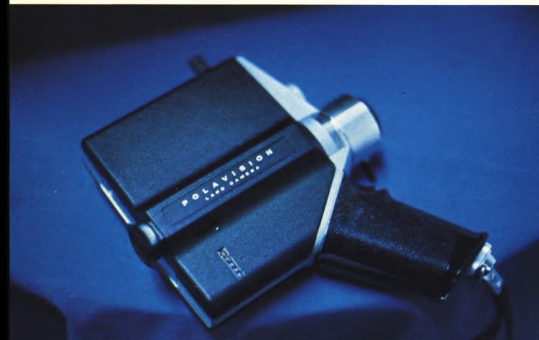
(LEFT) The Polavision camera is very lightweight and simple to operate, with two focus settings and automatic exposure control. Both camera and player are manufactured for Polaroid by Eumig. (RIGHT) Dr. Robert Doyle, President of Super8 Sound, beams happily as he tries the new camera. (BELOW LEFT) A mime goes through his act for stockholders at the meeting. (RIGHT) Film of the mime is shown on the player. (NOTE: The image on the screen appears a bit washed out, but this is due solely to slight overexposure of the still photograph. Polavision colors, when viewed on the player, are actually exceptionally rich.)
