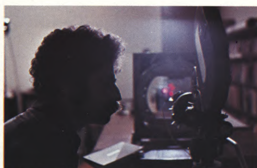
(LEFT) Rudnick filming into the laser. The vertical mount (center) was used for rotating various types of patterned glass and plastic. Viewing through the eyepiece was intermittent through a dense blue gel to cut down the laser intensity to a safe level. (CENTER) Director Dauber with set-up for filming into the laser, the beam of which can be seen in the center of the photo. (RIGHT) Another angle showing Dauber filming into the 5-milliwatt Helium-Neon laser. (BELOW LEFT) Lower segment of the balloon, with helium pipes leading into it, forms an interesting abstract pattern.
