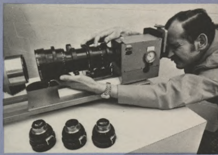
Proper flange focal seating, the infinity setting and the performance of an ARRI 35BL zoom lens is checked out by repairman Fabio Franco, on a special, factory equipped collimator.
