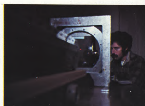
(LEFT) Rudnick filming into the laser. The vertical mount (center) was used for rotating various types of patterned glass and plastic. Viewing through the eyepiece was intermittent through a dense blue gel to cut down the laser intensity to a safe level. (CENTER) Director Dauber with set-up for filming into the laser, the beam of which can be seen in the center of the photo. (RIGHT) Another angle showing Dauber filming into the 5-milliwatt Helium-Neon laser. (BELOW LEFT) Lower segment of the balloon, with helium pipes leading into it, forms an interesting abstract pattern.
