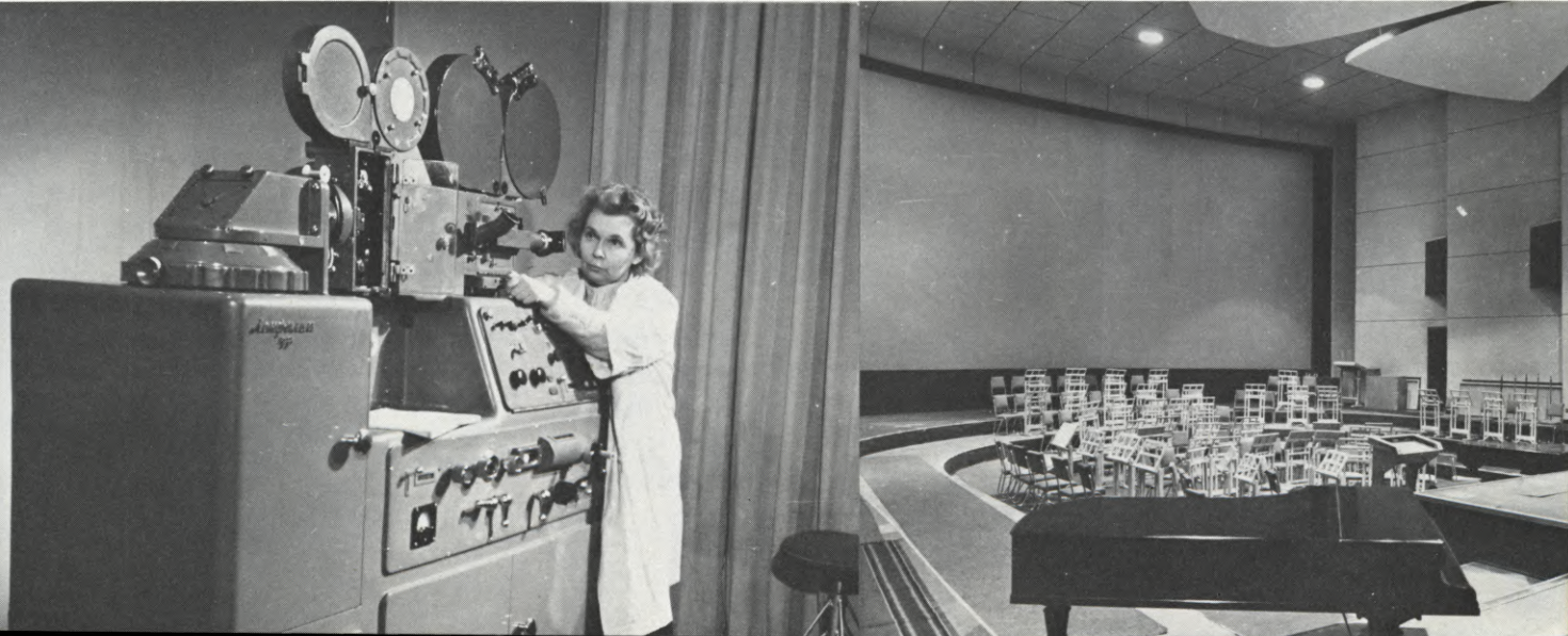
(LEFT) Special effects optical printer for 35mm film. Designed and manufactured at Lenfilm Studios, the optical printer is capable of performing 32 different operations. (RIGHT) Lenfilm's scoring stage for orchestra recording that can accommodate up to 60 musicians. The structure of the walls and ceiling makes for better acoustic characteristics.
