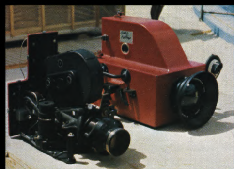
(LEFT) The specially modified (for underwater filming) Arriflex 2C camera, shown with the unique, highly sophisticated housing designed and partially built by Al Giddings, after it was discovered that no such equipment existed in the rental market. (CENTER) A front view of the camera. (RIGHT) One of the only ways of communicating underwater between director, actors and camera crew was to write on the back of the camera. The message here reads: "A bit faster through the hole."
