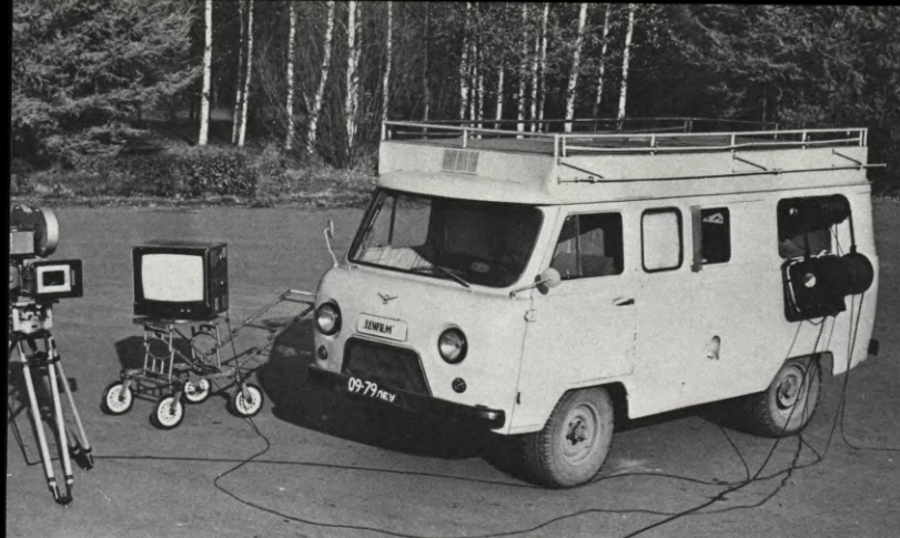
(LEFT) Video-monitoring system used on location involves a 3KSSU Cine-TV camera and monitor mounted on a collapsible trolley. The equipment is placed conveniently in a small bus and can be rigged up in a very short time for indoor and outdoor shooting. (RIGHT) A shot obtained by the electronic travelling matte process. The live action is shot in front of an infrared screen on a single, special-purpose film with the background exposed in optical printing steps by a narrow scanning beam.
