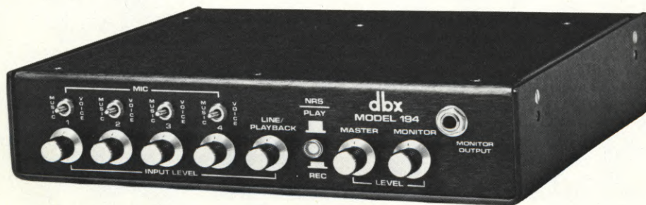
FIGURE 1 — The compact "dbx" unit is a boon to the sound recordist. By simply adjusting the level in such a way that the loudest peaks normally encountered do not exceed -10 dB, he can avoid overload of the tape caused by sudden loud sounds, and he is relieved of the necessity of riding gain.
