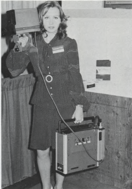
(LEFT) The new JVC 4400 portable 3/4" color video cassette recorder/player. (RIGHT) Is it a bird or a plane? Neither. It's the Gruber ENG-1 Cart that holds the video camera atop a cam-link head on an elevator column tripod. The lower part of the cart carries the CCU and recorder.
