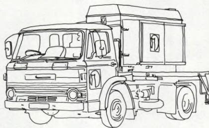
'D' Mount 250 amp - 120 V d.c. SILENT generator, shown left in working mode
