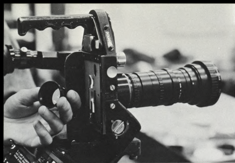
(LEFT) FIGURE 3 — When out in the field, use a magnifying glass to look through the ground glass attached to the aperture plate. (RIGHT) FIGURE 4 — The aperture plate should be checked for dust, hairs and emulsion build-up prior to the first shooting and, if possible, after each magazine change. To clean, use only a wooden orange stick, a clean soft handkerchief or chamois.
