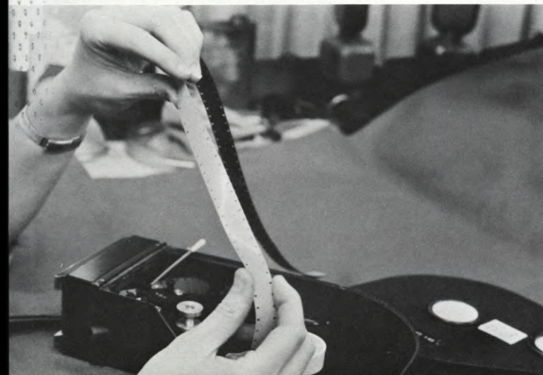
(LEFT) FIGURE 9 — To test for scratching, run a few feet of film through the camera, remove film from the takeup core and angle it so that the light will reflect off of it. (RIGHT) FIGURE 10 — Remove the magazine from the camera and also remove the takeup door. With a scissors, cut the film, one piece at a time, in the following places: Before and after the bottom takeup film gate, at the top and bottom on the pressure plate, before and after the top takeup gate. Examine each piece, looking for the origin of the scratch.
