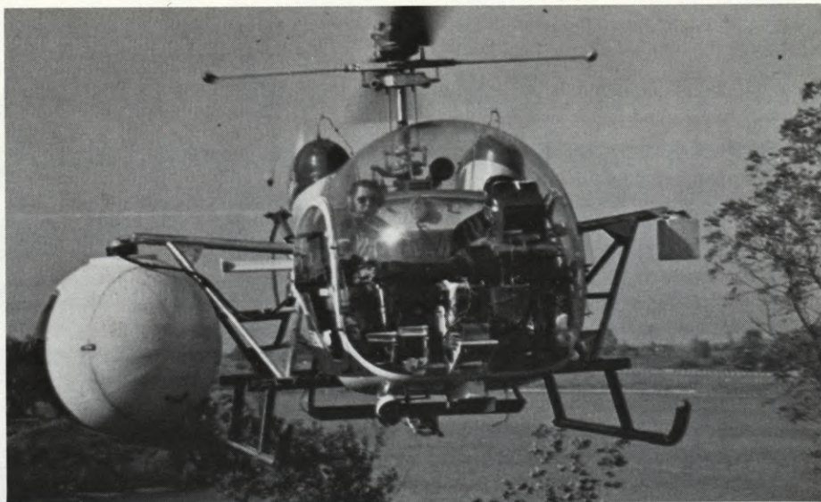
The Wesscam can be mounted under a helicopter, making possible a 360-degree pan, or side-mounted for easier landing (as shown here), in which case it permits a 210-degree horizontal pan. It can also tilt down 90 degrees and up 30 degrees above the horizon.
