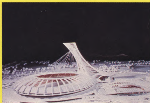
(LEFT and CENTER) Three-dimensional architectural models of the Olympic Park sports complex as it will look when completed. The rakish Tower will support, by means of cables, a retractable "lid" that will protect the field in inclement weather, but leave it open to the sky when the weather is fair. (RIGHT) The Olympic Stadium under construction. (BELOW) A three-dimensional model (LEFT) and two actual views of the Olympic village with its striking "half-pyramid" structures.
