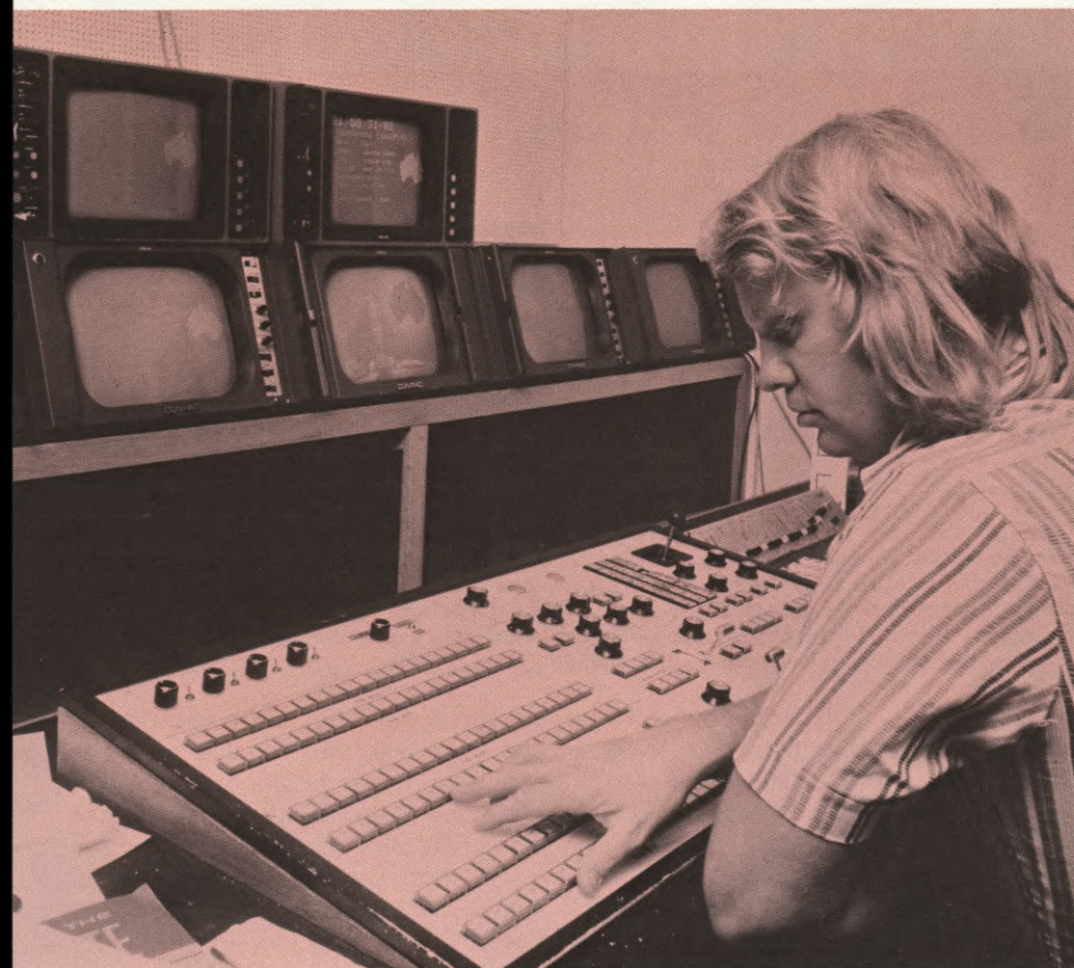
Enterprise Color Video Technical Director Brian Hicks works at the Richmond Hill Vision Mixer, which is EECO-controlled. The procedure of filming commercials in Panavision anamorphic for theater projection, and then electronically scanning the frame to extract the essentials for television has become widely accepted in Australia, since it saves money, while providing a top-quality result.
