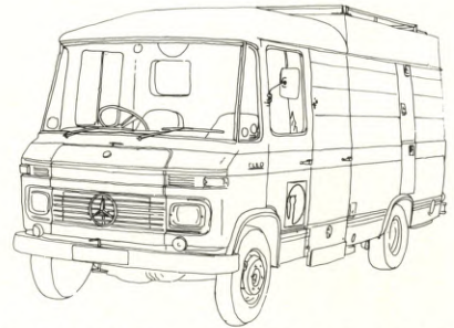
OWL II. Built-in 50 kVA - 120/240/415 V a.c. SILENT alternator with 311 cu. ft. of storage space (see below).
