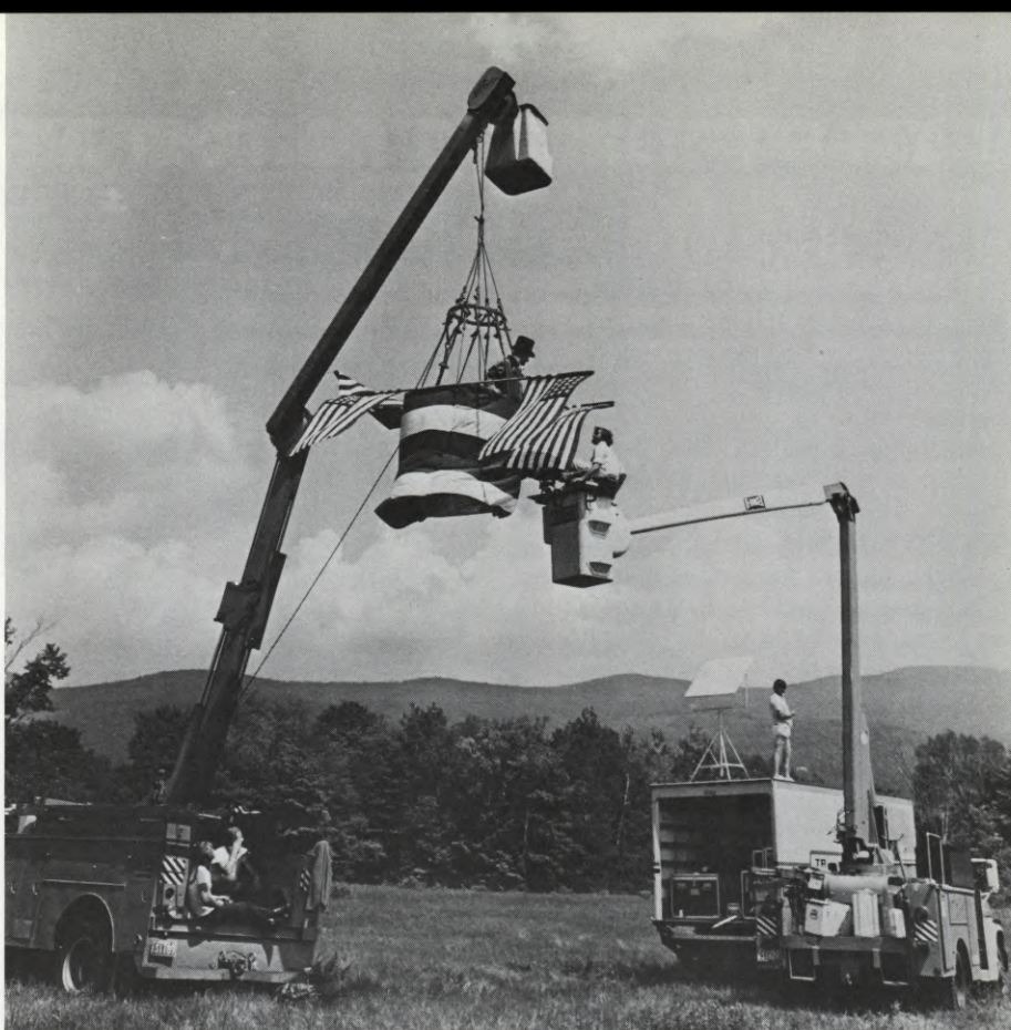
In order to simulate a balloon flight to shoot closeups of actor Peter Walker, the balloon's basket and the camera were suspended on two separate cherry-pickers, which moved in opposing directions to heighten the illusion of actual in-flight motion. Since the IMAX camera was used without a blimp, the dialogue had to be looped later.
