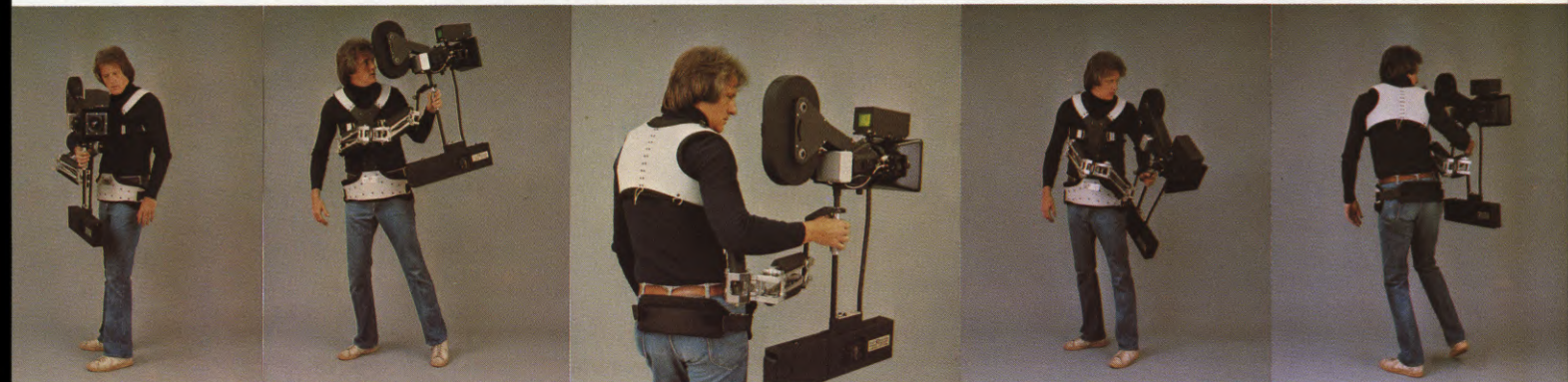
Garrett Brown demonstrates the amazing maneuverability of his invention, the revolutionary new STEADICAM-35. Whether held level or tilted up or down, the rig floats smoothly, like a miniature helicopter gliding at eye level. The operator can run with it, leap up steps and move swiftly over very rough terrain without the jerking and bouncing movements inevitable when ordinary hand-held cameras are used in such circumstances.
