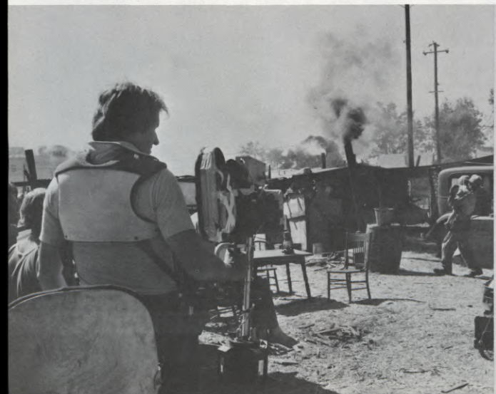
(LEFT) With the STEADICAM-35 "floating" from his body brace, Garrett Brown, inventor of the device, steps off camera crane platform and begins to move through the migrant camp. (RIGHT) Brown, with his STEADICAM-35 at the ready, sits in the bed of a pickup truck, as David Carradine prepares to drive it. The radically different new device effectively dampens the vibration and movement of practically any vehicle.
