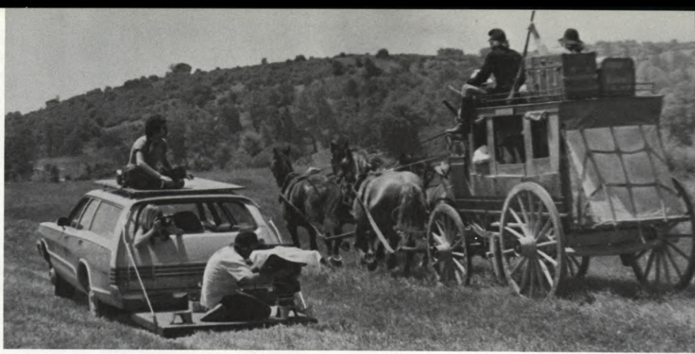
The Mac-Free camera car (with its special suspension) which had previously been used for shooting numerous car commercials and shorts, served perfectly to keep the IMAX camera in motion while pacing a stagecoach, a Model-T Ford or a steam locomotive. There are many such close, dynamic running shots in "TO FLY".
