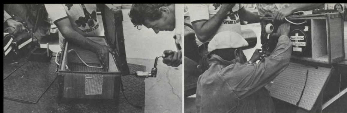
In an effort to get spontaneous action of the extras "living" in the migrant camp built for the film near Stockton, California, an Arriflex 35BL camera was installed in a suitcase with a port hole cut into the end. The camera operator, dressed to match the extras, was able to move inconspicuously among them and film their unstudied reactions. This lent an additional documentary touch to the sequence.
