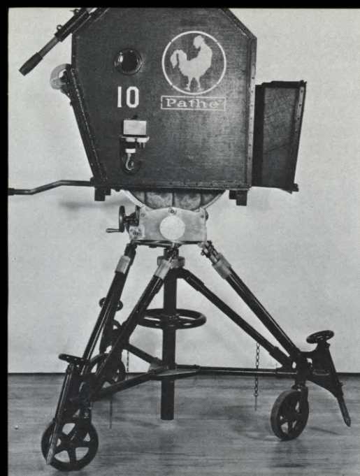
(LEFT) Early sound cameras required large, clumsy sound-muffling housings. Around 1930, the Pathé Camera and Sound Departments developed this design, credited to technicians L.E. Clark, Joe Wright, A.L. Domike and Ferol Redd. (RIGHT) A stockholders' meeting of the United Artists Studio in 1936. Top row, left to right: Charles Chaplin, Darryl F. Zanuck, Samuel Goldwyn. Seated: Mary Pickford, Joseph M. Schenck and Douglas Fairbanks.
