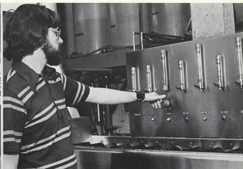
(LEFT) Most news stories are filmed on the scene and feature full visualizations, rather than merely "talking heads". (RIGHT) Because process VNF-1 for Eastman Ektachrome video news film 7240 (tungsten) eliminates the prehardener and neutralizer, WXYZ-TV has been able to shorten their film processing time to about 18 minutes.
