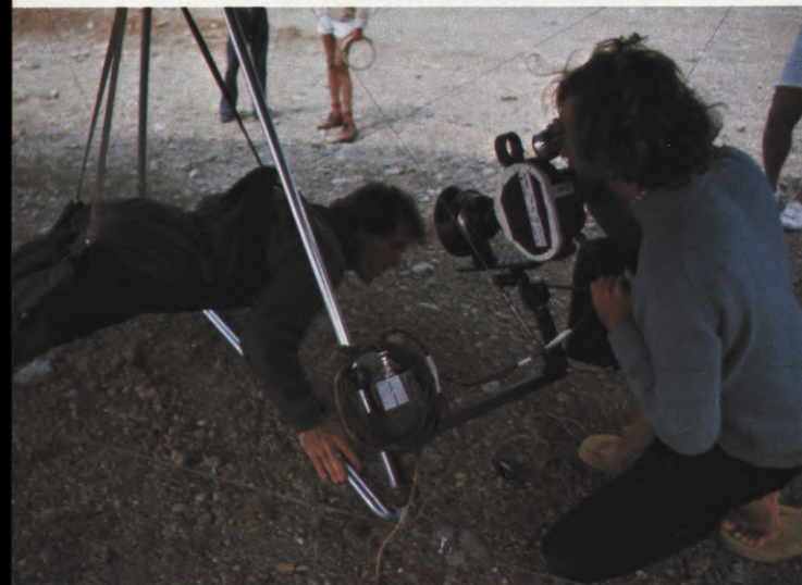
(LEFT) MacGillivray lines up a kite-mounted 100-foot Eyemo camera equipped with a 28mm lens in preparation for an inflight shot. The scenes shot from hang gliders were usually filmed at 32 frames per second in order to smooth out any slight unsteadiness. (RIGHT) There are no process or matte shots in "SKY RIDERS". The alternative, so that the principle actors would seem to be actually flying, was to suspend them from this giant crane in front of the camera.
