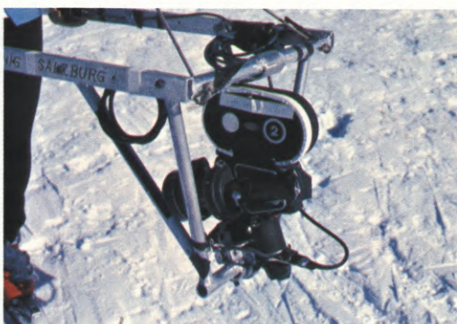
Herbie Raditschnig adjusts the Arriflex camera on the special mount with which he skis down the steepest slopes for filming purposes. The camera can be mounted in the front, in the rear or on the side. Raditschnig developed the rig about eight years ago and has used it for shooting innumerable commercials and travel films. For the Olympics film, he followed Austrian champion Karl Schranz down the Downhill run with it.
