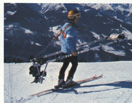
Herbie Raditschnig adjusts the Arriflex camera on the special mount with which he skis down the steepest slopes for filming purposes. The camera can be mounted in the front, in the rear or on the side. Raditschnig developed the rig about eight years ago and has used it for shooting innumerable commercials and travel films. For the Olympics film, he followed Austrian champion Karl Schranz down the Downhill run with it.
