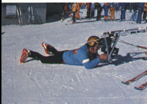
Herbie Raditschnig adjusts the Arriflex camera on the special mount with which he skis down the steepest slopes for filming purposes. The camera can be mounted in the front, in the rear or on the side. Raditschnig developed the rig about eight years ago and has used it for shooting innumerable commercials and travel films. For the Olympics film, he followed Austrian champion Karl Schranz down the Downhill run with it.
