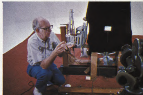
(LEFT) The Kodak Ektographic slide projector is mounted as the movable, controllable light source to illuminate the card. (CENTER) An adjustable mirror is attached to facilitate complete control of the light beamed onto the card. (RIGHT) Designer Ken Swartwout makes final adjustments of the device's mirror control. Extreme care was taken to keep the card in sharp focus and properly framed.
