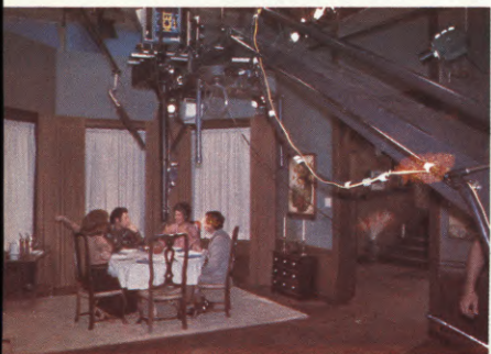
(LEFT) The Snorkel-B, with RCA TK-44, shooting on videotape at KCET. Here the lens-tube extension was used to get the camera high and out of the way of the steeply angled lights positioned on top of set walls. (CENTER) Shooting with Compact Video's Philips PCP-70 on Columbia Pictures TV Special, "COLUMBIA PICTURES 50th ANNIVERSARY". Camera traveled down one side of long table, across the end and up the other side to show name cards — all in a single take. (RIGHT) Shooting miniature domed city for "LOGAN'S RUN" at MGM Studios. Lighting by special effects expert L.B. "Bill" Abbott, ASC. Snorkel-B suspended more than 30 feet from Titan crane.
