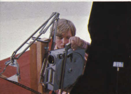
(LEFT) The Kodak Ektographic slide projector is mounted as the movable, controllable light source to illuminate the card. (CENTER) An adjustable mirror is attached to facilitate complete control of the light beamed onto the card. (RIGHT) Designer Ken Swartwout makes final adjustments of the device's mirror control. Extreme care was taken to keep the card in sharp focus and properly framed.
