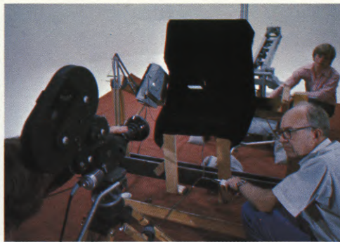
(LEFT) Director of Photography Jerry Hartleben sets up shoot, while the boom arm is activated through pulley mechanism. (CENTER) A closer look at the shooting setup. Note the vertical position of the frame movement in relation to the camera. (RIGHT) The zoom motor control is activated in order to produce the revolving movement of the card.
