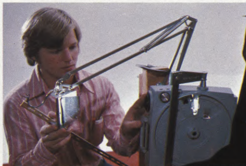
(LEFT) The Kodak Ektographic slide projector is mounted as the movable, controllable light source to illuminate the card. (CENTER) An adjustable mirror is attached to facilitate complete control of the light beamed onto the card. (RIGHT) Designer Ken Swartwout makes final adjustments of the device's mirror control. Extreme care was taken to keep the card in sharp focus and properly framed.
