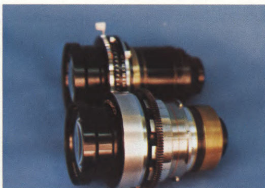
(ABOVE LEFT) The Zeiss 50mm, f/0.7 lens, shown in special focusing-mount (and with adjustable shutter blade removed). (CENTER) In front, the specially modified Zeiss 50mm, f/0.7 lens. Behind it, the lens before modification. (RIGHT) Zeiss 50mm f/0.7 lens with Kollmorgen adaptor, creating an effective focal length of 36.5mm (BELOW LEFT) Zeiss f/0.7 lens in special focusing mount. (CENTER) Lens with Kollmorgen adaptor — 36.5mm focal length. (RIGHT) The Cine-Pro T/9 24-480mm zoom lens, shown with J-4 zoom control.
