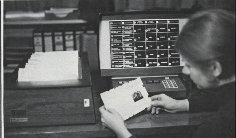
(LEFT) A sleeved card, which can hold trims up to two feet long (cut into three pieces, as shown here). (RIGHT) DataCode and Selector set-up, as used at the SMPTE exhibit for the simulated editing of "PSYCHO". For purposes of this demonstration storyboard scene sketches from the Film Classics Library book on "PSYCHO" were mounted on the cards. Appropriate buttons for selected scene characteristics, as indicated on the Overlay, light up when punched and will stay lighted until cleared by punching "Display Clear" button.
