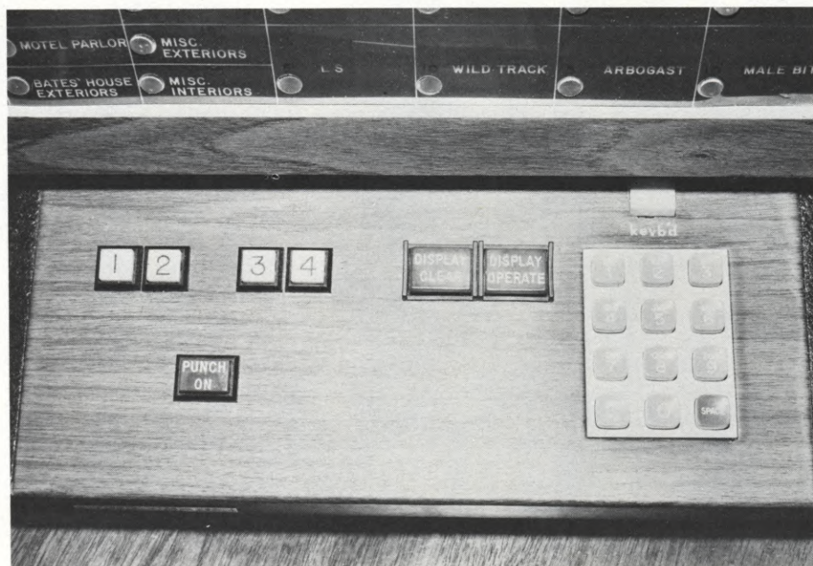
(ABOVE RIGHT) Keyboard in the DataCode set-up used for film editing. (BELOW LEFT) The DataCode editing set-up, showing Keyboard, Selector Tray and Punch. (RIGHT) Overlay for DataCode, programmed to a specific film, can be replaced with a different one in seconds. Overlay shown here is for "PSYCHO" and was used for demonstration at SMPTE exhibit. It was worked out by Robert Rowen, formerly of KEM Electronic, who serves as consultant to Intercraft in development of software for film industry application.
