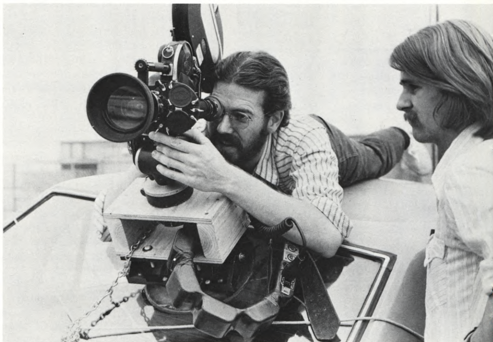
Ken Wheat, behind the Arriflex, prepares to shoot the Model T truck doing its thing for "STUCK ON THE SCREEN", while co-director Dave Madsen checks the action. Because the head of the Super-Grip did not allow for panning, a box was improvised that bolted onto the Super-Grip. Standard fluid head could then be mounted to permit panning and tilting. Like many of today's young film-makers, the crew of "STUCK" was fascinated by the 1920's Hollywood that swung wildly long before they were born. The film, which adopts a photographic style of the period, is thoroughly professional in every technical aspect.
