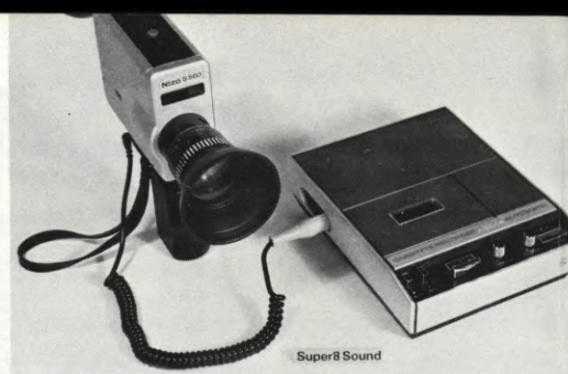
The Nizo S560 and Philips 2209 sync cassette recorder make an inexpensive and lightweight location rig. Camera and recorder may be crystal-controlled with the addition of external crystal boxes.
