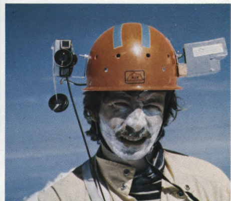
"Man from Mars" rig features a Bolex 233 camera mounted on Mountain Safety Research helmet, with cable release.
