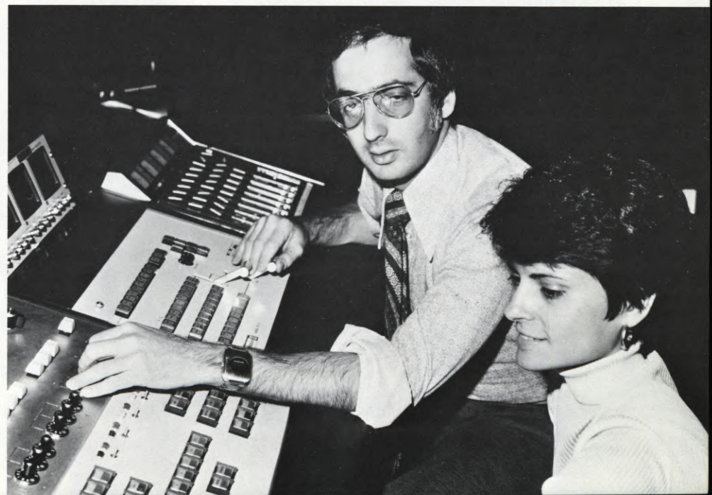
Phil Mancino shows Zeida Cecelia-Mendez how the National Video Center Color Corrector works. Her Super-8 footage of the International Dance Festival in Bulgaria, after transfer to 2-inch quad tape with automatic density control, image enhancement and color correction, resulted in a final quad tape of high broadcast quality.
