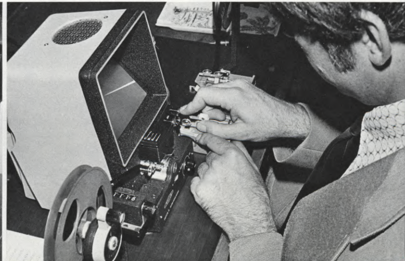
(LEFT) Film chain at KDUB shows the Kodak TVM100A Super-8 TV projector used with an RCA color TV camera. The projector's automatic threading has proved to be very reliable. (RIGHT) Editing Super-8 at KDUB, using the Wilcam sound editor and Bolex hot-splicer. Note the "seconds" counter on the left side of the editor. In 1972, KDUB-TV in Dubuque was the first station to announce a total commitment to Super-8 for both news and commercial production.
