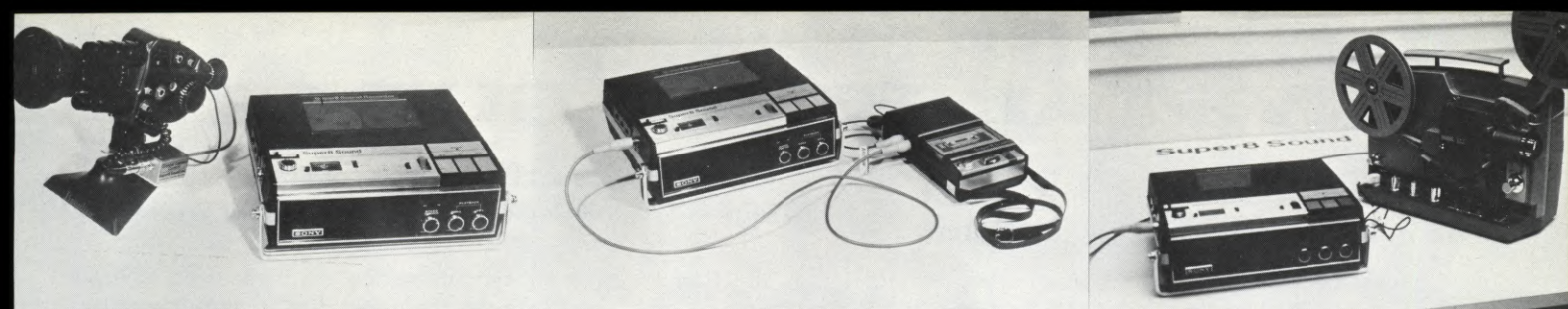
(LEFT) The crystal-controlled Beaulieu 4008ZM2 and the Super8 Sound Recorder make an extremely inexpensive crystal-sync location rig. More than 40 cameras which, like the Beaulieu, provide a sync signal output, may be used for cabled sync location work with this recorder. (CENTER) Very lightweight sync cassette recorders, such as the Super8 Sound Scipio, may be used to record sync sound. The Super8 Sound Recorder then automatically resolves these tracks. It can also transfer sound from pilotone sync recorders like the Nagra and Stellavox. (RIGHT) The Super8 Sound Recorder will synchronize with any projector equipped with a once-per-frame sync switch, for interlock screenings. It is shown here with the Bolex SM8 sync projector.
