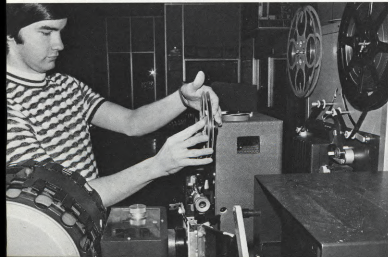
(LEFT) Film chain at KDUB shows the Kodak TVM100A Super-8 TV projector used with an RCA color TV camera. The projector's automatic threading has proved to be very reliable. (RIGHT) Editing Super-8 at KDUB, using the Wilcam sound editor and Bolex hot-splicer. Note the "seconds" counter on the left side of the editor. In 1972, KDUB-TV in Dubuque was the first station to announce a total commitment to Super-8 for both news and commercial production.
