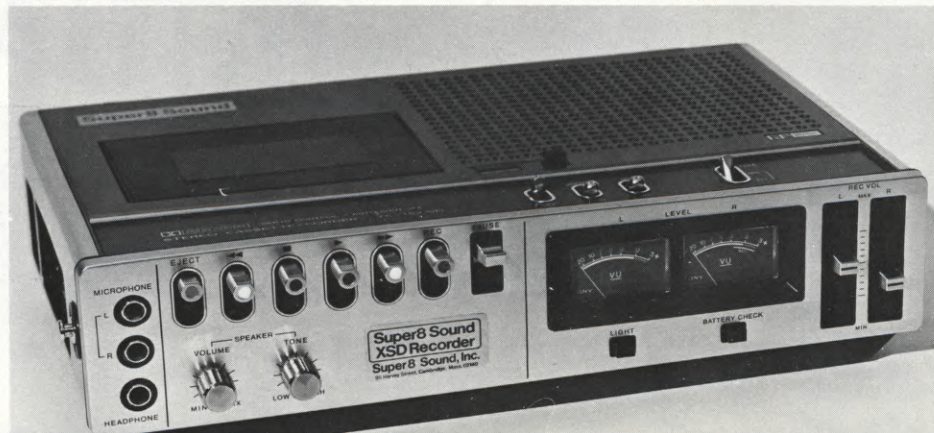
The XSD Recorder, based on the Sony TC153-SD cassette recorder with Dolby noise reduction circuitry, has internal crystal sync, as well as the capability to synchronize with cameras equipped with the standard pilotone output. A companion XSD Resolver is available for transfers of the sync sound to 16mm fullcoat magnetic film.
