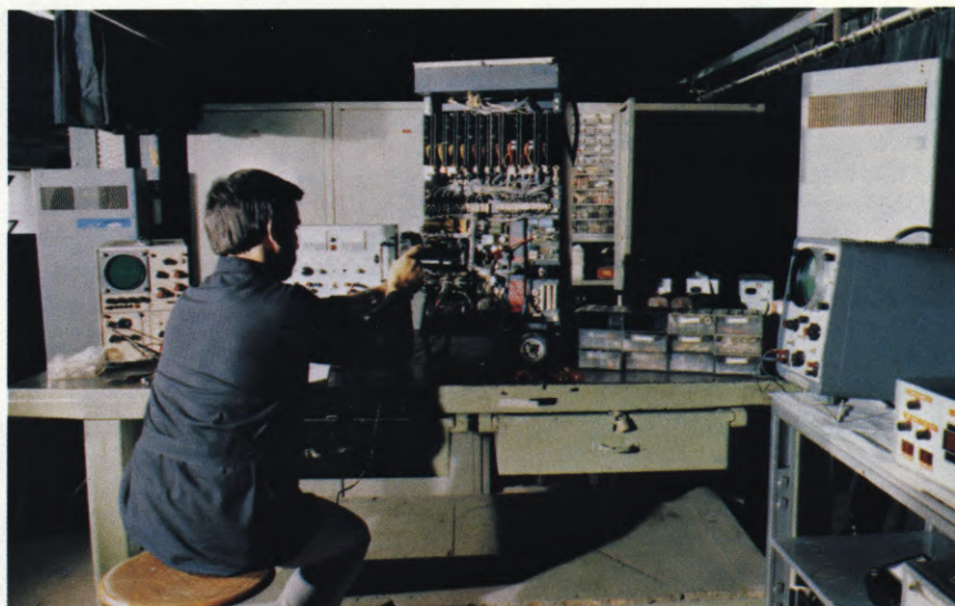
Technician at the QuartzColor Ianiro plant is shown at work on the company's new square-wave ballast. In prototype form, the unit (which will handle HMI lamps up to the 4000-watt model) is admittedly large and heavy, but may be left in place on the generator or equipment truck up to 100 feet from the lamp location. Production units should be smaller and lighter in weight.
