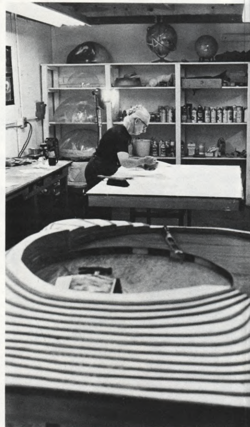
Sculptress Marion Connor develops models of Martian volcanic mountains. Foreground model shows topographic build-up made with fibreboard sections.
