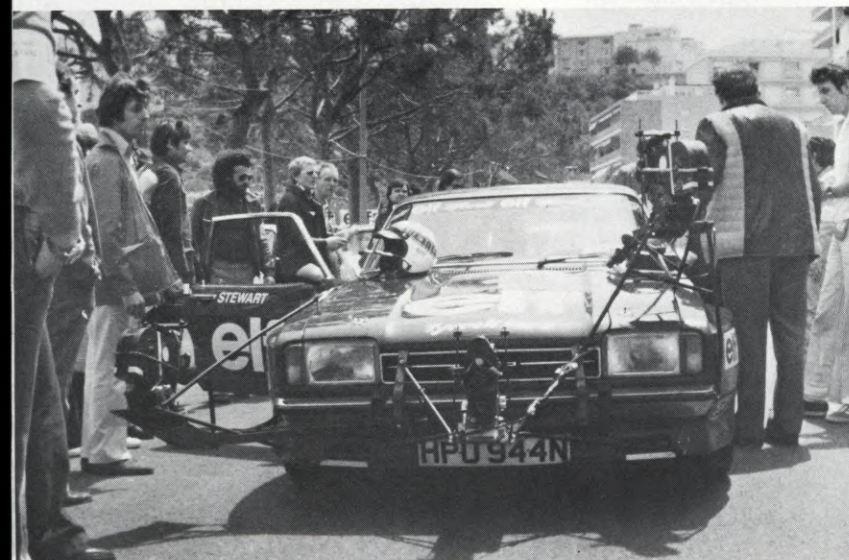
(ABOVE RIGHT) View of Stewart's Capri camera car showing unique mounting system for three external Eclair NPR's. A fourth NPR was mounted inside. (BELOW LEFT) A front end view of the car, showing the three externally mounted cameras. (RIGHT) Assistant cameraman Jim Williams adjusts camera mounted to film the right front wheel.
