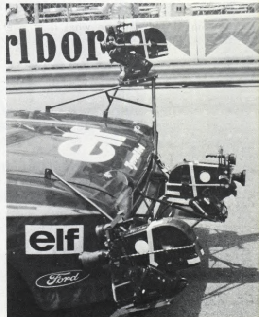
(ABOVE RIGHT) View of Stewart's Capri camera car showing unique mounting system for three external Eclair NPR's. A fourth NPR was mounted inside. (BELOW LEFT) A front end view of the car, showing the three externally mounted cameras. (RIGHT) Assistant cameraman Jim Williams adjusts camera mounted to film the right front wheel.
