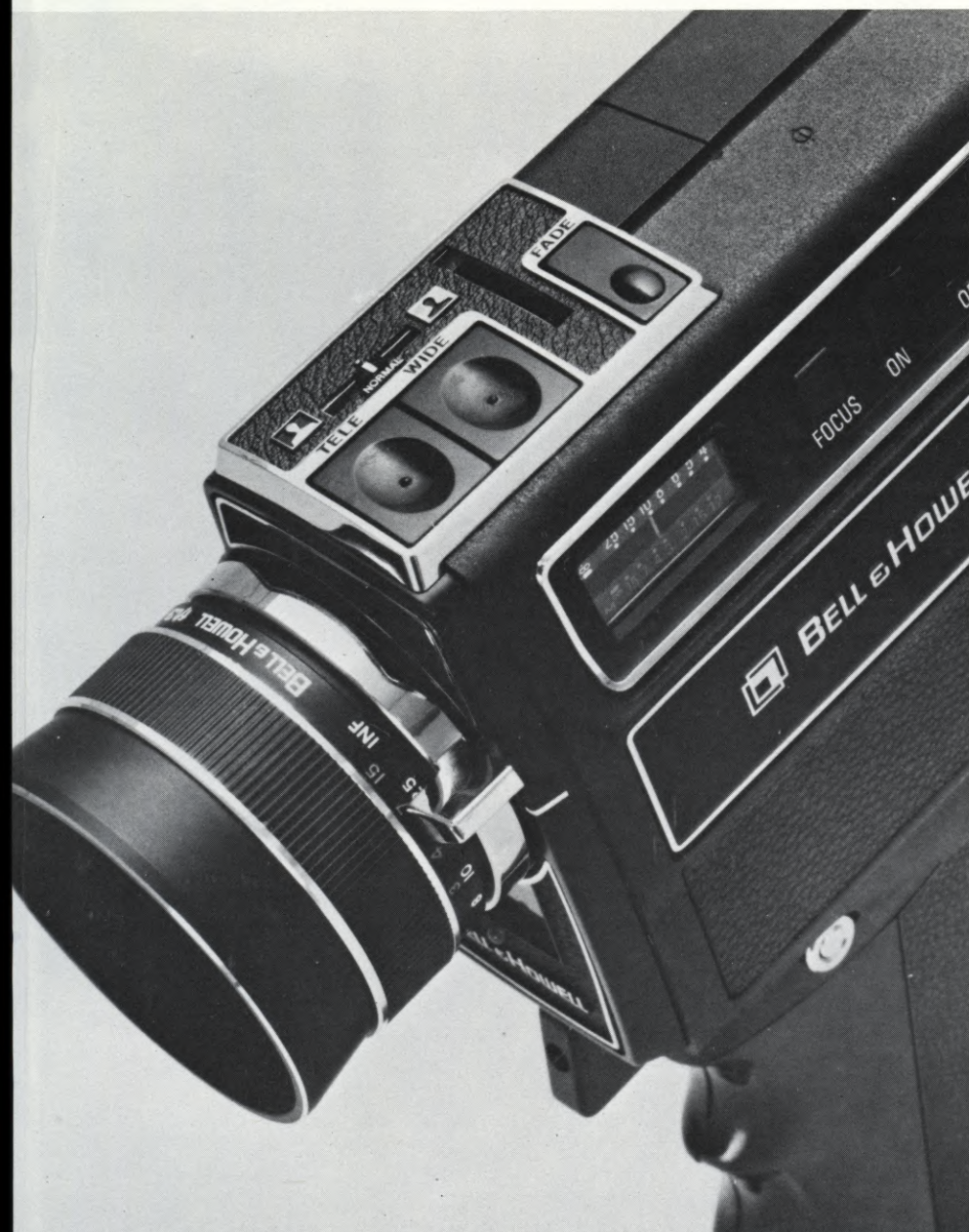
The full-time power zoom pushbuttons, fade-out and fade-in button and contrast control switch are all conveniently clustered at the top front of the camera body where they can be easily reached and operated by the fingers of either hand. Positioned below the lens, the red cue light provides subjects with a visual signal when the camera is operating.
