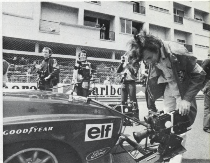
(ABOVE RIGHT) View of Stewart's Capri camera car showing unique mounting system for three external Eclair NPR's. A fourth NPR was mounted inside. (BELOW LEFT) A front end view of the car, showing the three externally mounted cameras. (RIGHT) Assistant cameraman Jim Williams adjusts camera mounted to film the right front wheel.
