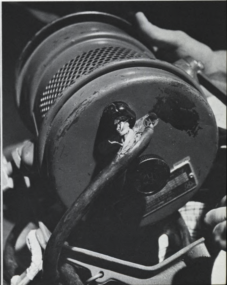
(LEFT) Safety harnesses should be doubly connected to the grid when gaffers adjust lights, and hands should be gloved. (RIGHT) Abused electrical cables are highly dangerous and should be replaced at once. The film industry considers it standard procedure to scout locations before shooting, so that there will be no unpleasant production surprises, but how many producers scout safety hazards, as well?
