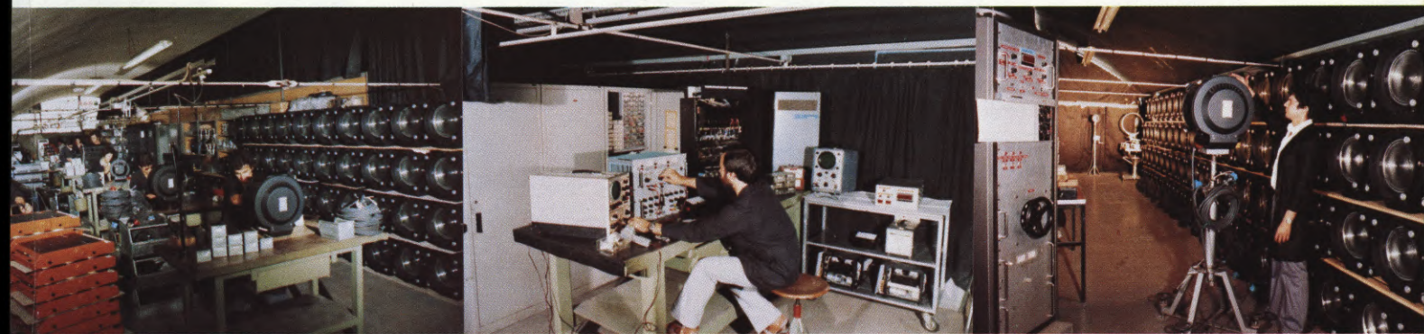
(LEFT) The Electrical Assembly Department. (CENTER) The TEsting Room, where electronic equipment is used to test various elements. (RIGHT) The Measurement Room, where the light curve of each lamp is scientifically measured and recorded on graph paper by the apparatus on the left. Each individual lighting unit is subjected to multiple tests and measurements before being approved for shipment from the plant.
