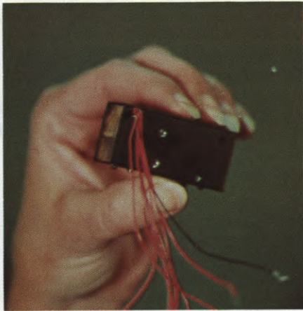
This tiny device is the resolver which might be called the "heart" of the new system. It is part of a simple, low-cost conversion kit which fits onto the theatre projector.
