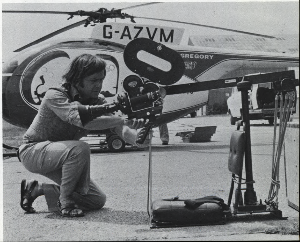
(LEFT) The original one-piece base-plate of the mount has been replaced by a two-part plate which enables the SKYMOUNT to fit into the floor of the Jet Ranger 206A and B, as well as smaller helicopters, such as the Hughes 269 and 300. (RIGHT) To be comfortable with the SKYMOUNT, the cameraman is seated on a foam-filled seat pad, complete with backrest, seat belt and footrest. (BELOW) Cameraman/Designer Mervyn Wilson installs Arriflex camera on the SKYMOUNT. Assembly of the mount takes only a few minutes, including installation in the aircraft.
