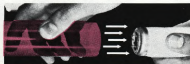
Sleeves are applied directly to the tube.
