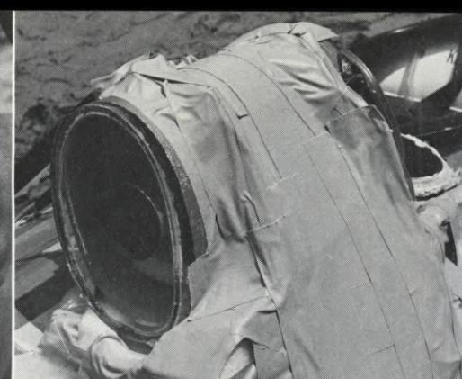
(LEFT) The tiny GZAP, magazine-loading 16mm camera, developed as an aircraft gun camera during World War II and refined for other remote uses since then, was used to get point-of-view shots from the kayaks. Although a 5.7mm lens was available, the 10mm was the lens almost always used on this camera. (CENTER) Suitably miniaturized battery for driving the GZAP camera. (RIGHT) The GZAP camera secured inside a waterproof housing with glass front and mounted on the front of the kayak.
