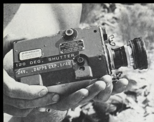
(LEFT) The tiny GZAP, magazine-loading 16mm camera, developed as an aircraft gun camera during World War II and refined for other remote uses since then, was used to get point-of-view shots from the kayaks. Although a 5.7mm lens was available, the 10mm was the lens almost always used on this camera. (CENTER) Suitably miniaturized battery for driving the GZAP camera. (RIGHT) The GZAP camera secured inside a waterproof housing with glass front and mounted on the front of the kayak.
