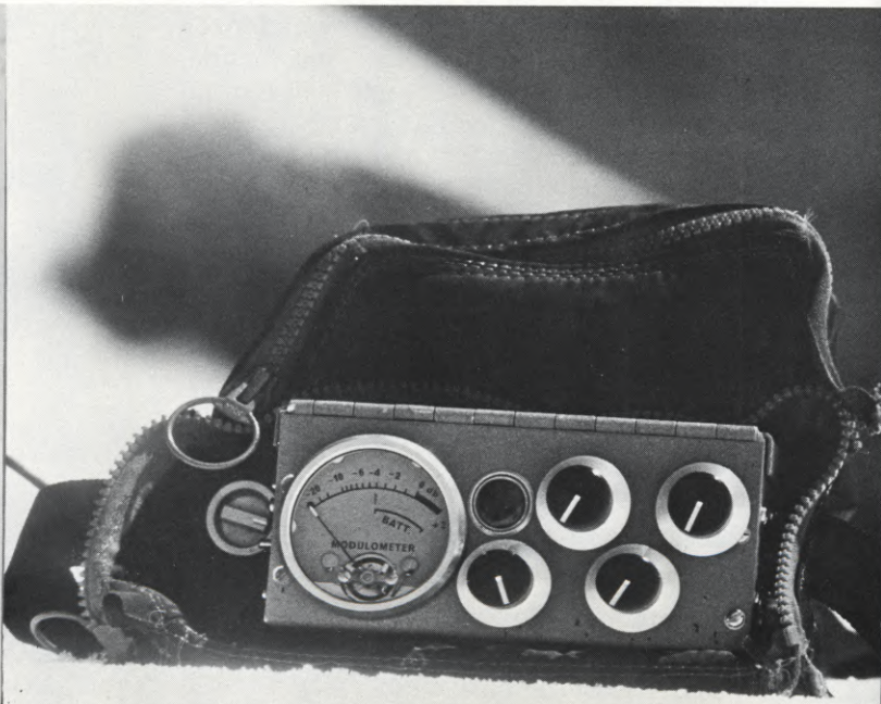
(LEFT) The highly miniaturized Minitek Mixer designed and built by soundman Peter Pilafian and used by him on "THE EIGER SANCTION" and other difficult assignments. The upper compartment contains a Nagra SN miniature recorder and spare tapes. The switch on the left is for LF equalization. (RIGHT) Waterproof carrying case is made from nylon backpack material. The two small switches on top control the SN recorder.
