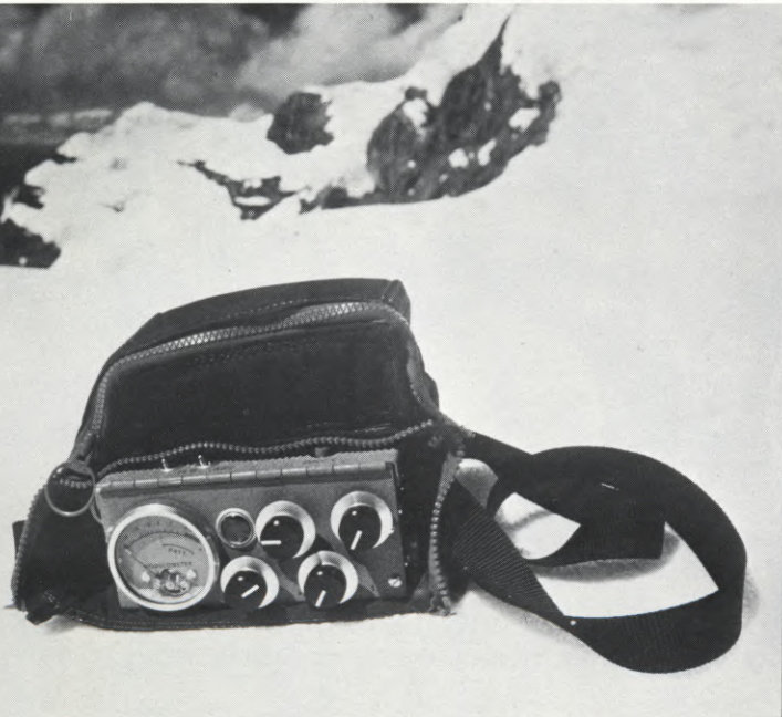
(LEFT) The highly miniaturized Minitek Mixer designed and built by soundman Peter Pilafian and used by him on "THE EIGER SANCTION" and other difficult assignments. The upper compartment contains a Nagra SN miniature recorder and spare tapes. The switch on the left is for LF equalization. (RIGHT) Waterproof carrying case is made from nylon backpack material. The two small switches on top control the SN recorder.
