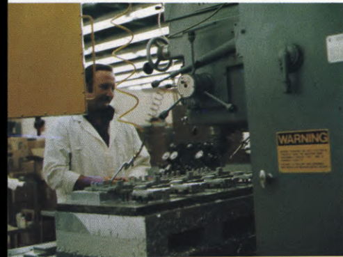
(LEFT) One of the tape-controlled milling machines simultaneously producing 10 high-precision identical parts for the CP-16R. (CENTER) Check-out equipment for lenses which must be fully tested and completely checked out before delivery to user. (RIGHT) An environmental test chamber.
