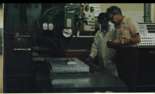
The Sound Test Room (LEFT) was specially designed for total isolation, and is used to set standards for the 35mm and 16mm "quiet" CP cameras. (CENTER and RIGHT) The tape-controlled, high precision, milling machines. Cinema Products has three machines of this type which produce the high precision, interchangeable parts for the 35mm and 16mm cameras.
