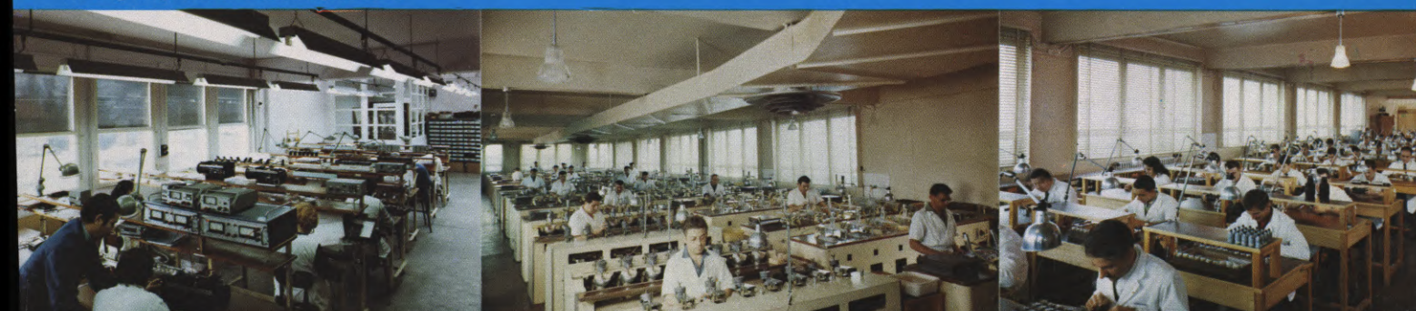
(LEFT) Electronics assembly. Electronic components activate motorized zoom lenses and automatic Iris lenses. (CENTER) The optical polishing department, where the most critical operation in the manufacture of lens elements takes place. At least a year is required to train a technician to perform the more critical polishing operations. (RIGHT) Optical assembly, the last major manufacturing step.
