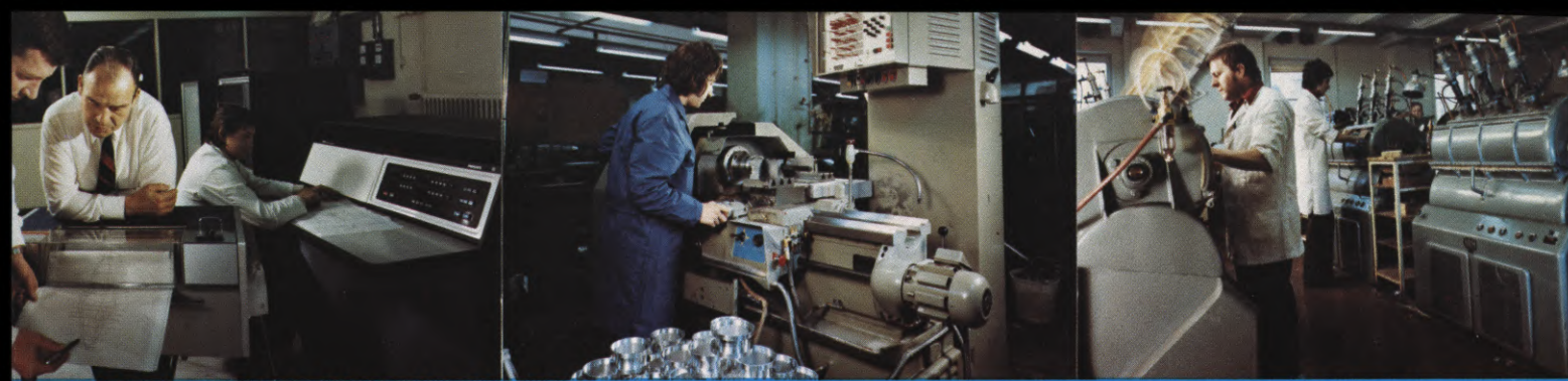
(LEFT) Mr. Corbasson (Manager) and Mr. Masson (Technical Director) are shown discussing a ray tracing of one of the latest optical designs in the computer room of the Angenieux optical design department. The company creates all of its own programs for the computer. (CENTER) Operator checks on a tape-controlled machining process. (RIGHT) The optical grinding department, where the elements of a lens begin to take shape.
