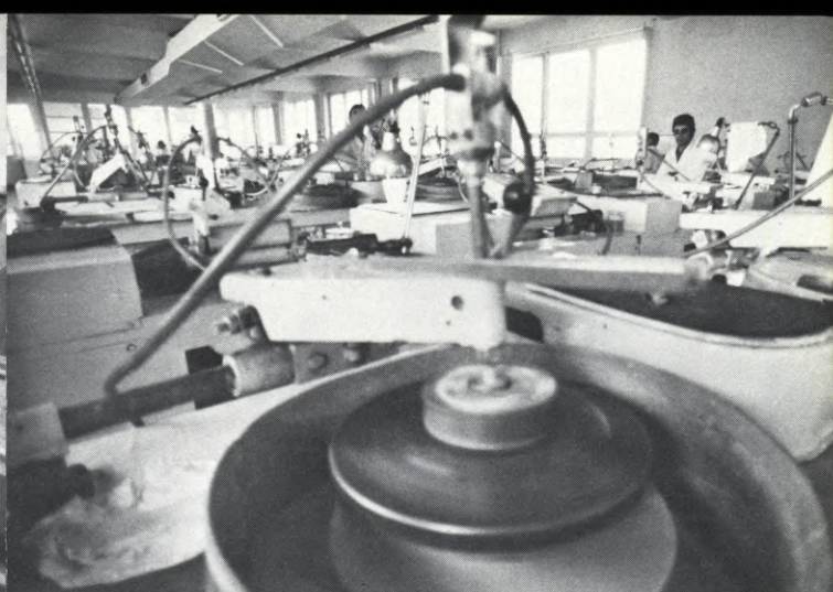
(LEFT) Rough blanks for zoom lens elements await grinding and polishing. (RIGHT) After rough grinding, which takes about a minute, the potential lens elements are sent along for polishing, which may take one or more hours. An individual polishing machine (foreground) works on several elements at once. Polishing is a very critical phase of lens manufacture.
