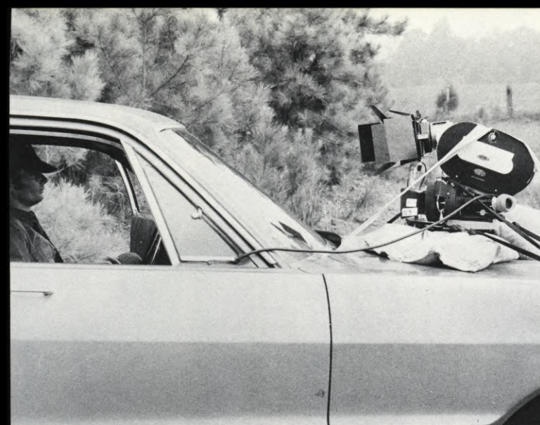
When shooting the auto chases, it was necessary to mount cameras on various parts of the cars. Jim Latham and Bert Bertolami did wonders with Super-grips and Century arms, plus, of course, a bit of gaffers tape. As the cars gradually got wiped out, it became necessary to use a car for several different purposes. One day a car might belong to a moonshiner and the next day it would be a police car. A quick repainting job did the trick.
