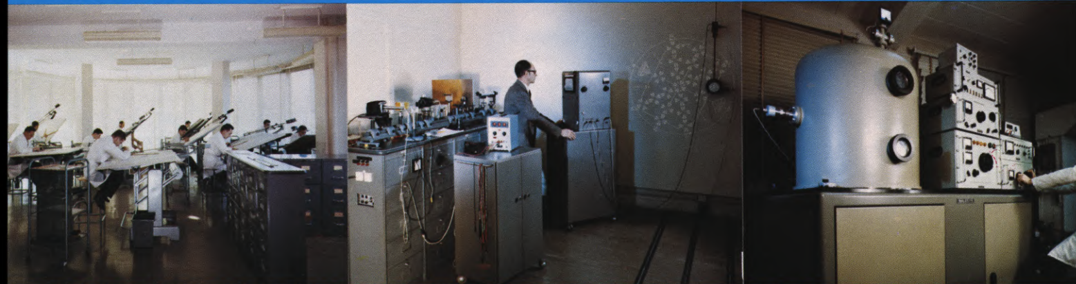
(LEFT) The Angenieux drafting department is located in a pleasant glassed-in rotunda, with an inspiring view of the surrounding countryside. (CENTER) Mr. Dimler (Director of the Optics Lab) is shown making MTF measurements in his facility. (RIGHT) Multi-layer coating equipment, employed to apply successive layers of magnesium fluoride and other chemicals to lens elements in order to minimize the degree of reflection.
