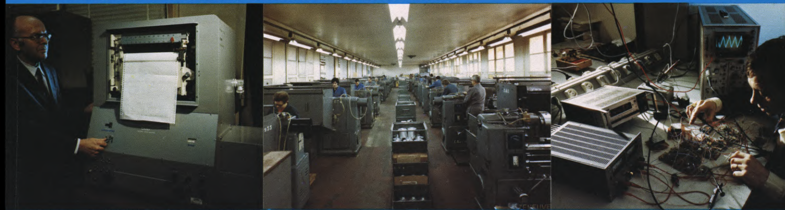
(LEFT) Mr. Michalet (Manager of Quality Control) is shown running dichroic measurements with a spectrophotometer. At the Angenieux factory, 80 out of the 700 employees are engaged in various aspects of quality control. (CENTER) Row on row of sophisticated equipment in the machining department. (RIGHT) A corner of the electronics lab. Electronics figures prominently in the manufacture of TV lenses that have servo-controlled zoom focus and Iris.
