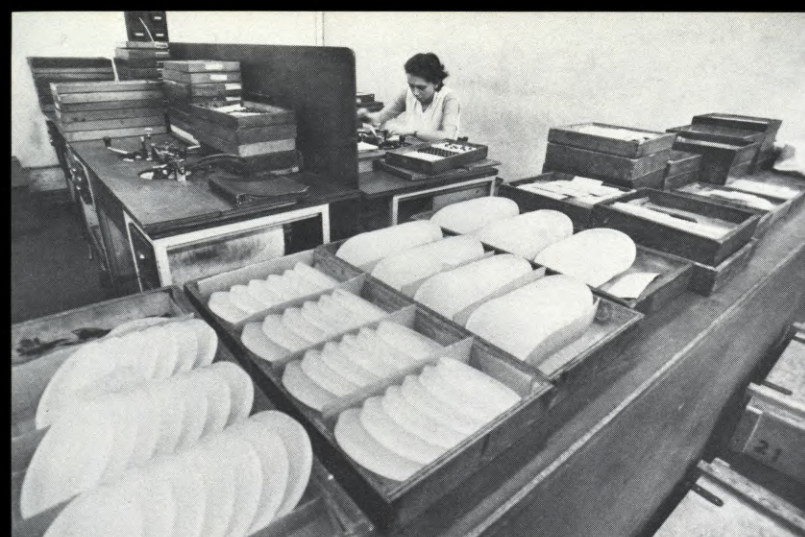
(LEFT) Rough blanks for zoom lens elements await grinding and polishing. (RIGHT) After rough grinding, which takes about a minute, the potential lens elements are sent along for polishing, which may take one or more hours. An individual polishing machine (foreground) works on several elements at once. Polishing is a very critical phase of lens manufacture.
