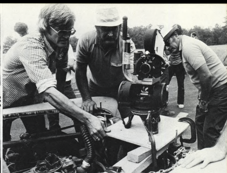
When shooting the auto chases, it was necessary to mount cameras on various parts of the cars. Jim Latham and Bert Bertolami did wonders with Super-grips and Century arms, plus, of course, a bit of gaffers tape. As the cars gradually got wiped out, it became necessary to use a car for several different purposes. One day a car might belong to a moonshiner and the next day it would be a police car. A quick repainting job did the trick.
