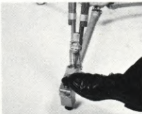
Simple foot-actuated lever raises dolly off wheels for positive locking action.
