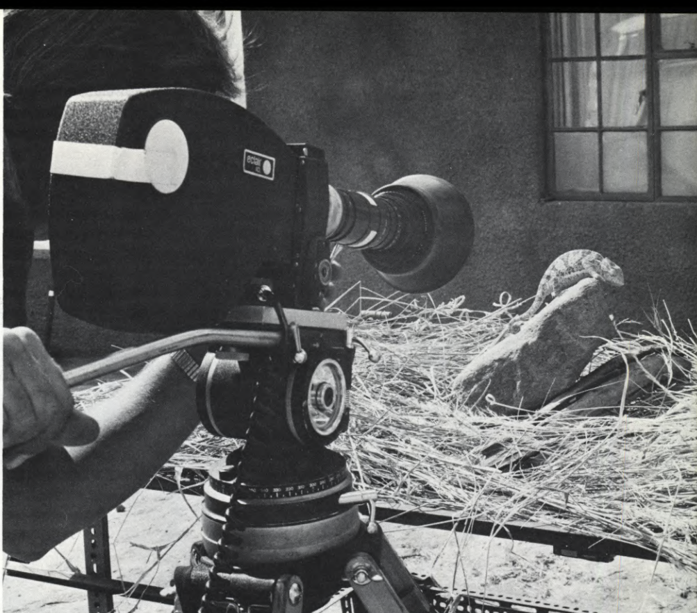
Mander uses the Eclair ACL, with 12mm-to-120mm Angenieux lens to film a chameleon on a rock. Cameras used were Eclair NPR and ACL, specially adapted by Eclair in England to the Super-16 format. Besides standard zooms, lens complement included a variety of Kinetals from 12.5mm to 90mm, plus 300mm and 500mm Macro-Kinoptic lenses. Two Nagra IV and two Nagra SN recorders were used.
