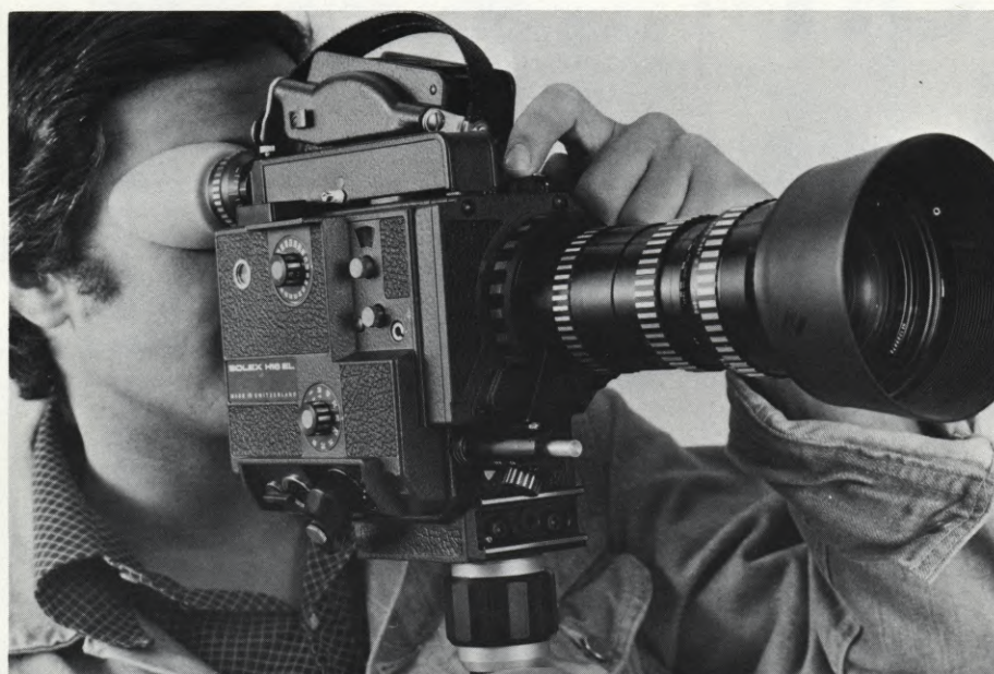
(ABOVE) FIGURE 1 — On the Bolex H-16 EL camera, the silicon light measuring cell is automatically moved out of the aperture by depressing the release button and moved back in by depressing the cell lever. (BELOW LEFT) the Vario-Switar 16mm-100mm lens, with fully automatic diaphragm adjustment and power zoom.
