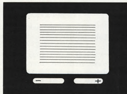
FIGURE 3 — Silicon cell measures shaded area (about 35% of the total field). Two red lighted diodes below indicate correct aperture when they are of equal brightness.
