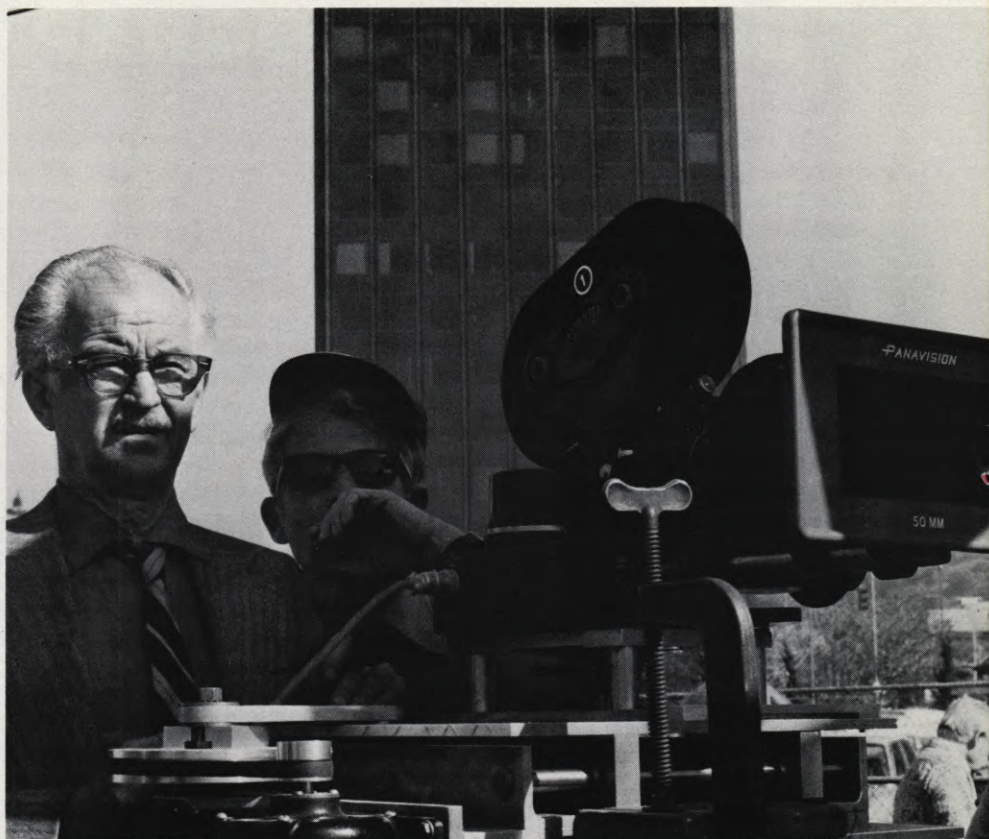
Alexander Golitzen shown with Panavision-adapted Arriflex camera mounted on a special shaker device worked out by Director of Photography Phil Lathrop and Lou Ami, head of Universal's machine shop. The shaker provided programmed vertical and horizontal movement in pre-conceived erratic patterns. The degree of vibration could be widely varied and a particular set of movements could be repeated precisely, if needed.
