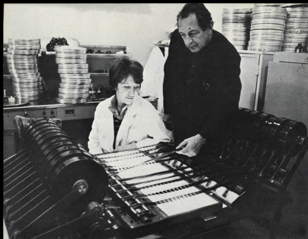
Separate film strips arranged in a multiple synchronizer for the cutting of a multi-image film. The Varioscopic process, as developed at Mosfilm, permits several images which are inter-related dramatically, to be presented simultaneously in varying shapes upon a 70mm (5-perforation) frame, thus permitting a wide variety of creative possibilities.
