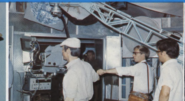
(LEFT) Hand-holdable "1 KCWP" 70mm mirror-reflex camera, which is often used for 3-D filming, exposing two adjacent images on each 70mm frame. It is a 12-volt-powered camera with 160' shutter, mounting a 200' magazine and weighing 16 pounds. (CENTER and RIGHT) Crew working on the science-fiction feature "SOLARIS".
