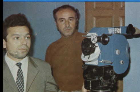
(LEFT) Hand-holdable "1 KCWP" 70mm mirror-reflex camera, which is often used for 3-D filming, exposing two adjacent images on each 70mm frame. It is a 12-volt-powered camera with 160' shutter, mounting a 200' magazine and weighing 16 pounds. (CENTER and RIGHT) Crew working on the science-fiction feature "SOLARIS".
