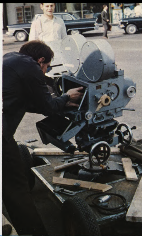
(LEFT) Newsreel cameraman, using hand-held camera with zoom lens. (CENTER) "Checking the gate" is the same in all languages. The camera shown is the non-reflex 70mm camera, Type 70 KCK, which is capable of exposing film at frame rates up to 90 fps. Note the geared head. Rear handle operates pan; side handle operates tilt. (RIGHT) Newsreel cameraman operating news camera mounted on tripod with telephoto lens.
