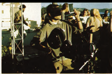
(LEFT) Cameraman Nick Nizich, with 16mm Arriflex camera on an equatorial mount during the eclipse shoot in Costa Rica. (CENTER) Assistant cameraman Bob Libby views eclipse during mid-annularity through two exposed sheets of 4 x 5" black and white film to protect his eyes from the infrared rays of the sun. (RIGHT) Libby checking camera position during annular eclipse. Motor drive for the equatorial mount is visible on the right.
