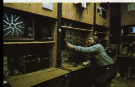
(LEFT) Dan Sandin processing a computer-generated image in his Chicago laboratory by means of his Image Processor. As the Image Processor is fed by a patch from the camera, the tuning knobs on each module permit control of value changes during the processing of the signal. (CENTER) Live subject in Sandin's lab, from whose features an unlimited number of altered images can be computer-generated. (RIGHT) Sandin and his "black wall of spaghetti."
