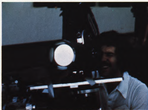
(LEFT) "Eclipse King", Dr. Donald Menzel led the eclipse expedition to Costa Rica last December. (CENTER) Nick Nizich shooting the eclipse with a Micro-line Sun Filter, which reflects the ultra-violet, visible and infrared solar energy in order to protect the cameraman's eyes. It also keeps heat out of the telescope optics. These filters have density factors of 5.0-0.001 percent transmission and the one shown here was the 4-1/2" size. (RIGHT) Expedition photographers seen setting up for an early morning shoot at Playa Flamingo.
