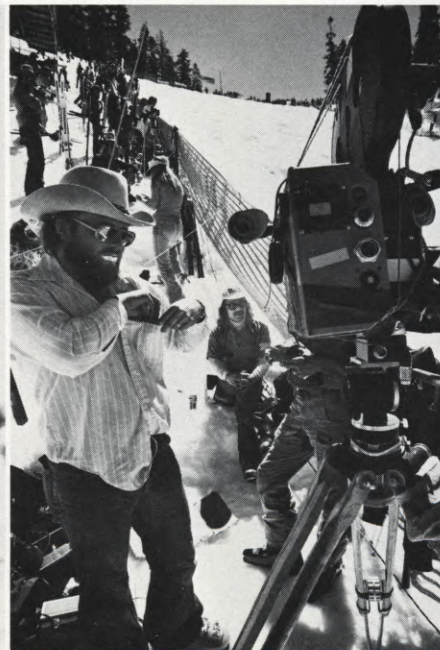
(LEFT) A Locam high-speed instrumentation camera (built by Redlake Corporation) is mounted next to Bolex Rex V camera with gaffer tape so direct cuts can be made from normal 24-frame footage to slow-motion footage of the same scene. (RIGHT) The improvised “dual camera” on tripod is readied for action on snow platform built halfway down the Freestyle Mogul course.
