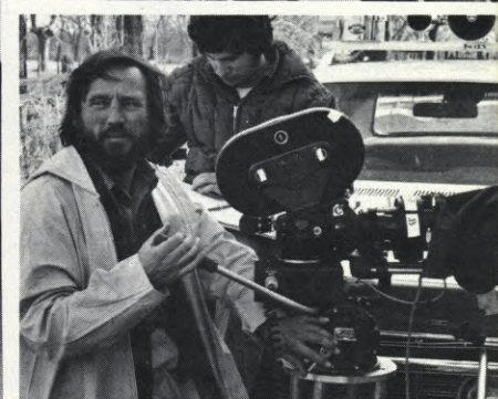
Zsigmond checks out the Arri 35 2C mounted on platform extending from front of police car.
