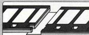
Ordinary splice leaves a bump on the film and a jump on the screen.
