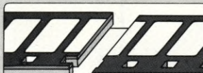
Ordinary splice leaves a bump on the film and a jump on the screen.
