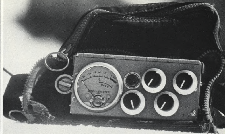
Prototype of the Minitek Mixer, developed by Soundman Peter Pilafian especially for this excursion. The upper compartment contains a miniature Nagra SN recorder and spare tapes. Switch on the left is LF equalization. The makeshift waterproof carrying case was fabricated from nylon backpack materials. The two small switches on top control the Nagra SN recorder.
