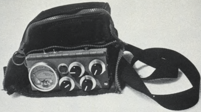
Prototype of the Minitek Mixer, developed by Soundman Peter Pilafian especially for this excursion. The upper compartment contains a miniature Nagra SN recorder and spare tapes. Switch on the left is LF equalization. The makeshift waterproof carrying case was fabricated from nylon backpack materials. The two small switches on top control the Nagra SN recorder.
