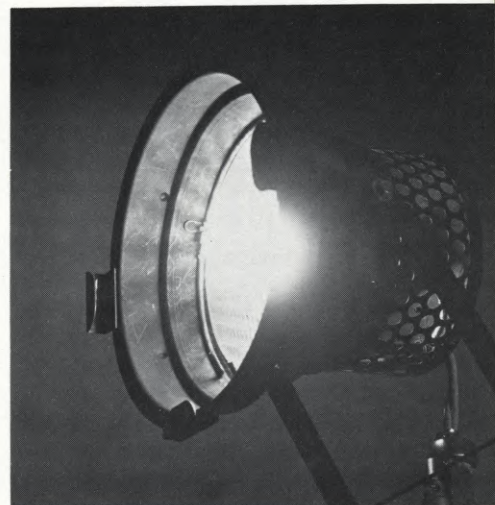
(ABOVE) New Art Bodkins Daylight PAR-64, 1000-watt long-life lamp under test. Globe employs a 3200°K GTE/Sylvania capsule, transferred to 6000°K by optical coating of reflector. (BELOW) Art Bodkins 250-watt Xenon Sun-Scout, designed for TV news cameramen. Contains a convertible reflector system from 6000°K to 3200°K. Operated on 30-volt battery.
