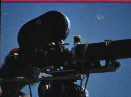
(LEFT) Special machinings and adaptation to side-mounted motor base were necessary to mount the maximum 3200mm lens. (CENTER) Arri 35BL made possible a complete sync-sound unit kept in readiness. Cameraman and soundman could grab entire unit and run. (RIGHT) Soundman Kevin Courtts places Audio Radio Mike on the late Francois Cevert. Nagra S allowed voice and background to be recorded separately for balancing later.
