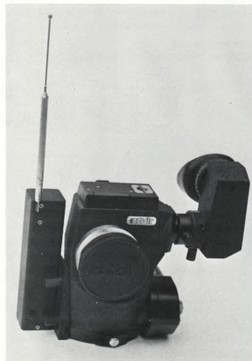
FIGURE 1—Miniature transmitter of the Cameraman's Remote Start/Slate RS/S-2 System, shown attached to body of Eclair ACL camera. Each time the camera is started, the automatic bloop light in the camera flashes several frames and radio transmits bloop tone to receiver at the recorder.
