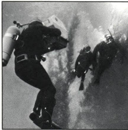
J. Barry Herron using Arri 16S with 400 foot magazine inside Birns & Sawyer underwater housing.
