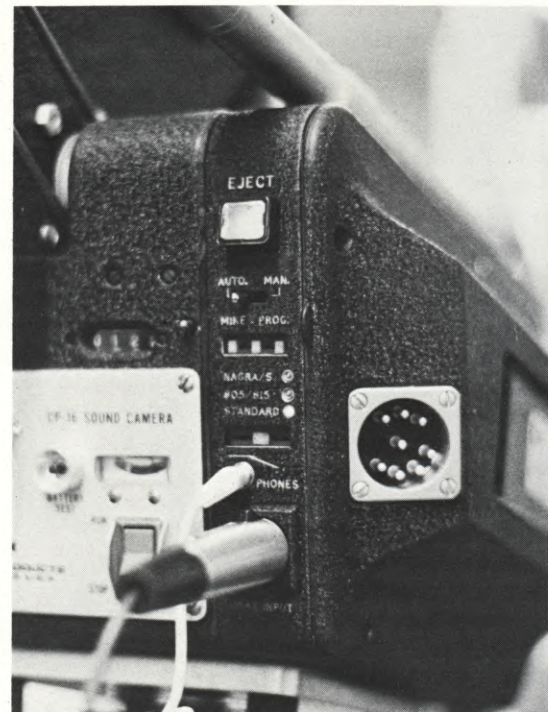
Rear view of "sandwich" between CP-16 camera motor housing and battery compartment, showing pilot lights for microphone program and interlock warning system.
