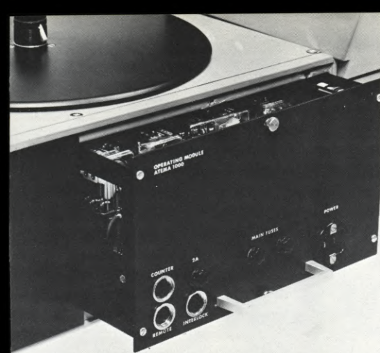
The Operating Module contains all of the electrical components and controls all mechanical functions of the table. It contains relays in plug-in sockets, plug-in boards for variable speed control and trim points.
