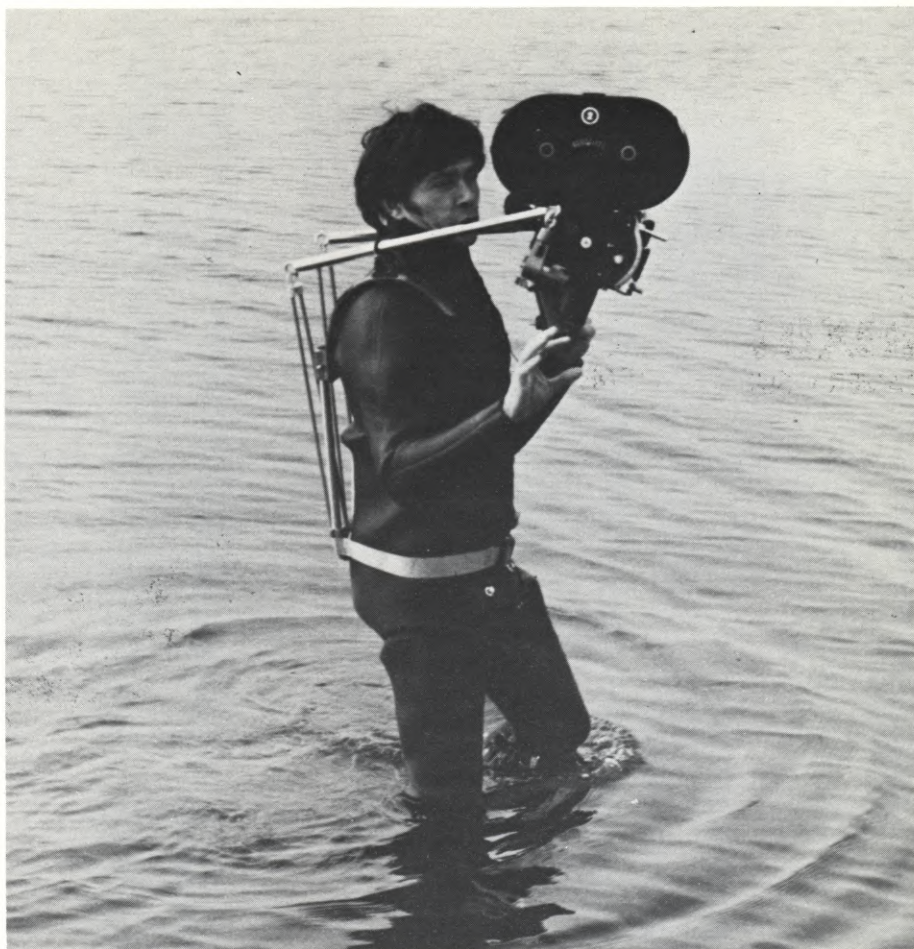
Camera, supported by the Fleximount, is not rigidly fixed, as with most other mounts, but "floats" for easy panning or tilting. Salient feature is that it is considerably more comfortable than conventional mounts, relieving a great deal of the strain inherent in hand-holding heavy cameras. Fleximount's "universal" design makes it adaptable enough to support several types of cameras of differing configurations.
