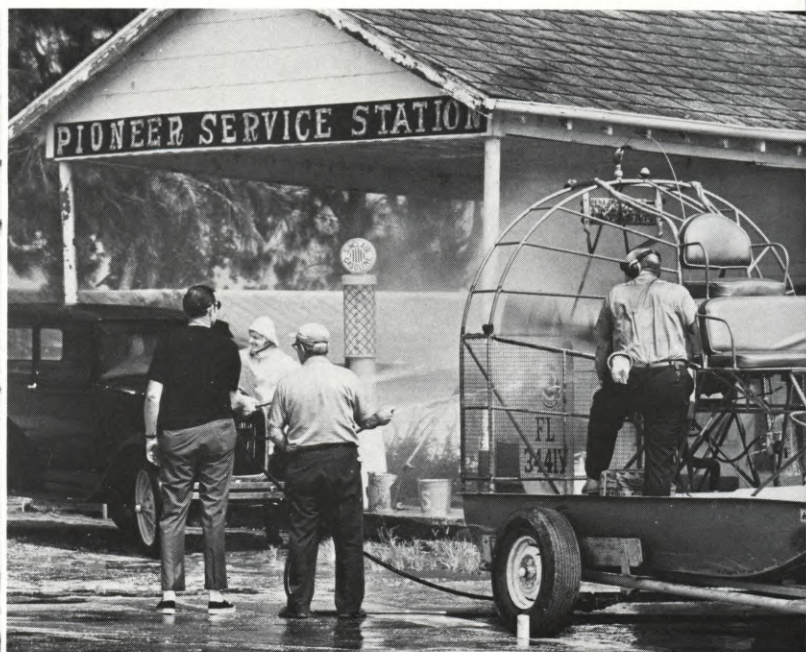
(LEFT) Cinematographer Dave Englund makes final check on scene through ortho viewing glass. Note ortho filter in matte box, used to lend a chalky appearance to the whites, an effect characteristic of ortho-chromatic rendering. (RIGHT) Water played into the airstream of a wind machine produced a very realistic horizontal rain effect.
