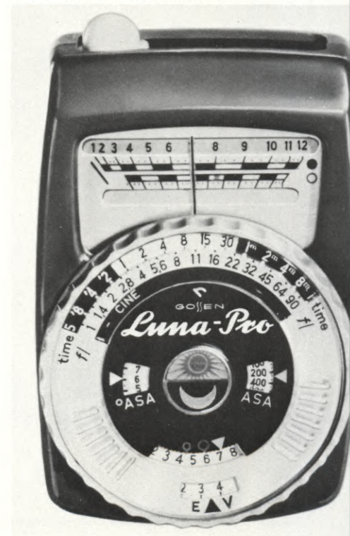
FIGURE 2—Reflective type meter, which also includes incident light capability.
