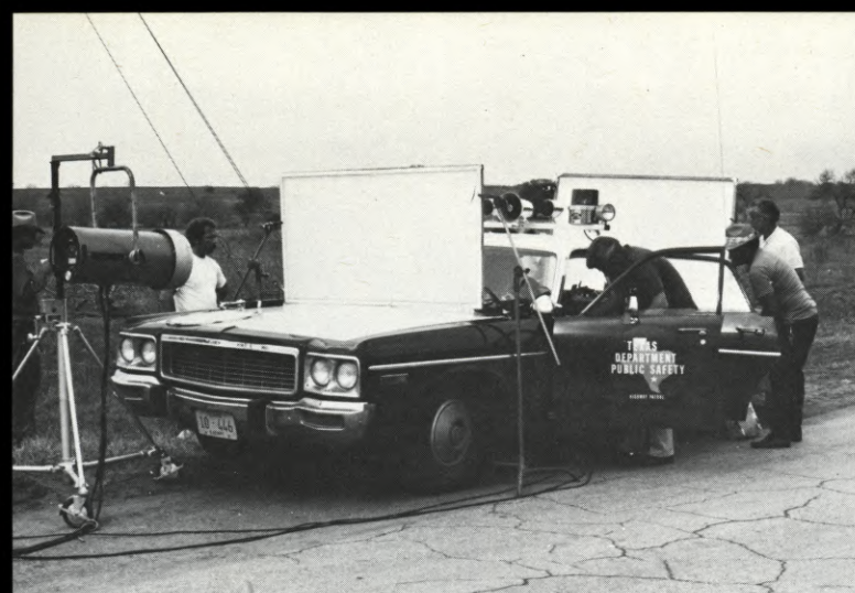
(LEFT) Xenotech Sunbrute lamps are beamed through mylar diffusion screens to provide soft fill-light for scenes shot inside the stationary car. These small, highly efficient lighting units (which are no longer produced) obviated the necessity of taking along cumbersome conventional Brute arcs on difficult locations. Cinematographer Zsigmond had previously used them to good advantage in shooting tricky sequences for "DELIVERANCE".
