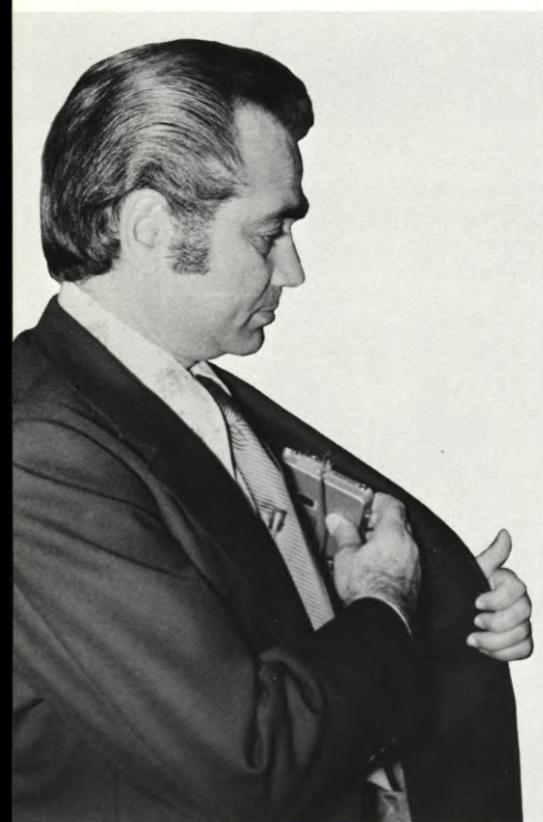
(ABOVE LEFT) The tiny Nagra SNN recorder weighs one pound, one ounce and fits in the palm of the hand. Developed by Stefan Kudelski, it features crystal-sync and automatic level control, plus optional mini-radio start-stop and bloop accessory. (BELOW LEFT) Self-contained SNN unit fits neatly into an actor's pocket. (RIGHT) The "ELDORADO" perambulator-type recorder originally accommodated 3,000 feet of 35mm mag-stripe film, running at 45 feet per second and could run one hour without reloading. It was later adapted to 17-1/2" sprocketed full-coat and then to 1/4" tape.
