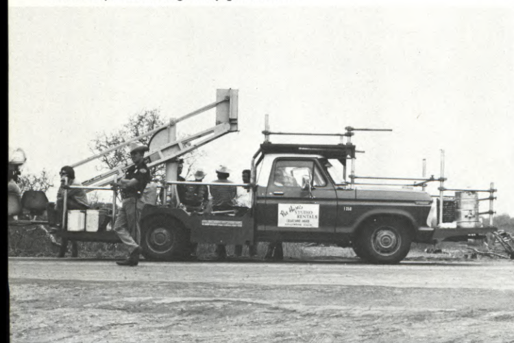
(LEFT) Unique camera car designed and operated by Pat Hustis features a 12-foot boom and an array of batteries concealed in various areas of the truck's body, so that banks of lights can be run without resorting to usual battery cart. (RIGHT) Throw-switch on side of truck, which permits quick conversion from 120 volts, for conventional lamps, to 36 volts needed to run xenon arcs. About 70% of lighting on film was run from these batteries, eliminating noisy generator.
