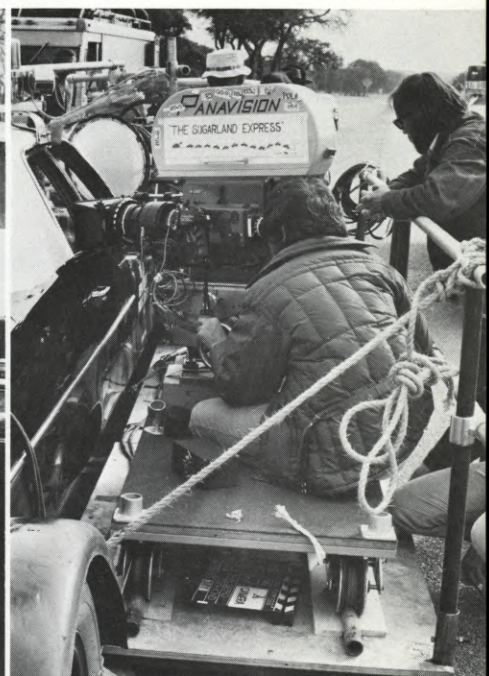
(LEFT) Zsigmond checks camera mounted on platform on the front of police car. (RIGHT) Outrigger platform on side of vehicle permits dolly shots with Panavision R-200 camera moving from rear to front window, while the car is in motion driving down the road. These shots were made prior to the arrival of the Panaflex on location, which would have made things a bit easier.
