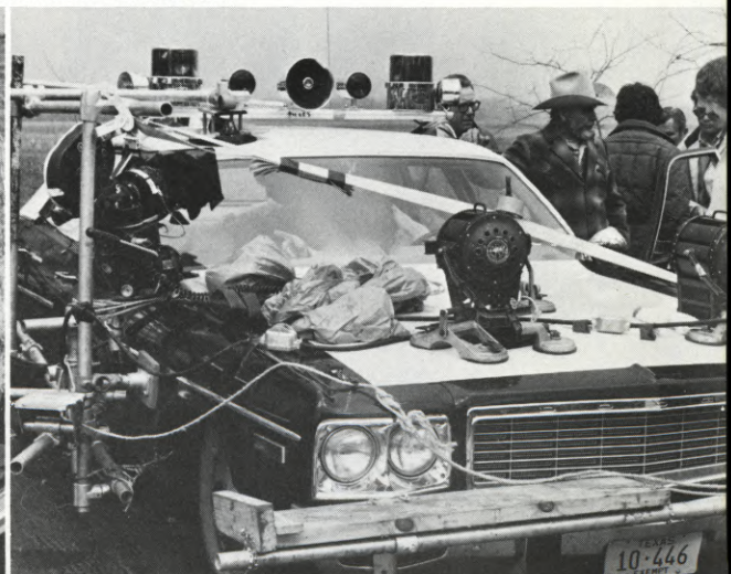
(LEFT) Zsigmond and McLean check rigging of lights and remote camera on the hood of a car. (RIGHT) Police car rigged within an inch of its life with lights and remote camera held on by suction-cup devices and other supports. Since the main action of "THE SUGARLAND EXPRESS" is a prolonged chase, most of the action takes place inside the car, necessitating the design and rigging of many complex mounts such as this.
